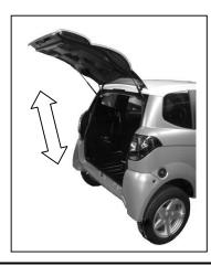
Lower the tailgate three fourths of the way and release it. Make sure that it is correctly locked
