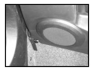
Pull the unlocking control located under the dashboard to the left.
