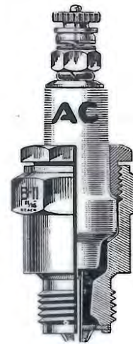
The A.C. Titan plug in part section.
