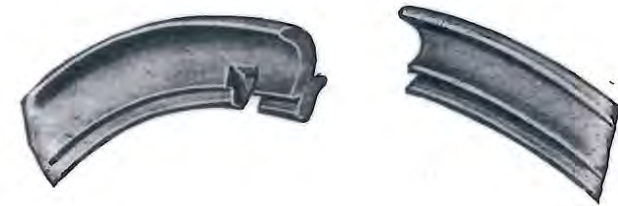
The two ends of the detachable spring flange showing slot into which the end of the lever is fitted for removal.
