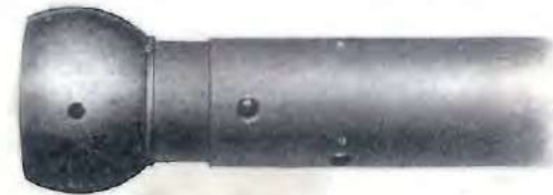
The torque tube ball joint which should be lubricated weekly via the Tecalamite nipple on top of the ball joint housing.
