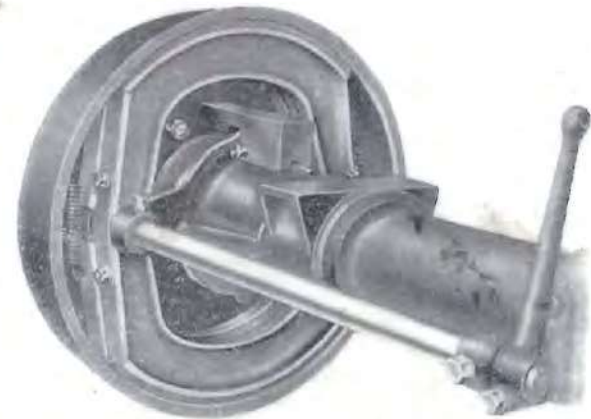
The brake assembly with dust shields removed showing special tool in position and engaging with the castellations in the hub locking ring.
