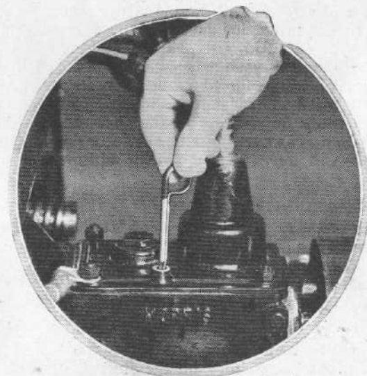
The rear end of the gearbox, showing the oil filler and some adjacent components.
