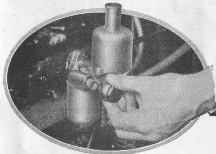
The filter is released by unscrewing the hollow hexagon screw attaching the petrol pipe to the float-chamber lid. Note that the open mouth of the filter faces outwards.
