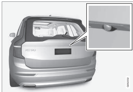
Location of the rear Park Assist Camera (generic illustration)
