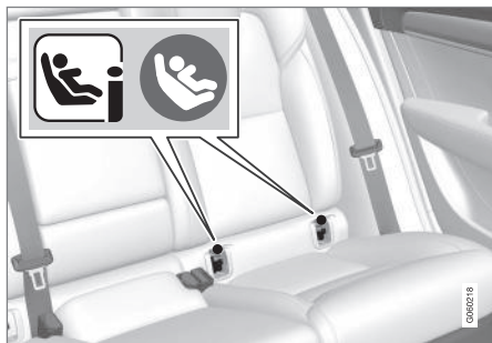
Location of the ISOFIX/LATCH anchors
