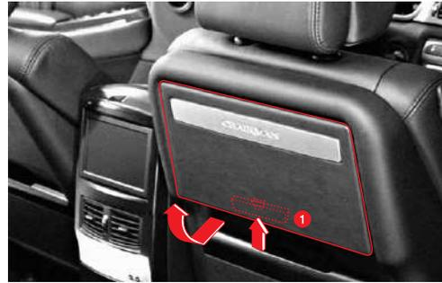
A table is on the rear of the passenger's seat for temporary jobs while the vehicle is stopping and putting on goods for rear seat occupants.
