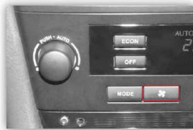
When in AUTO mode, press the fan switch and the MANUAL indicator will lit.
