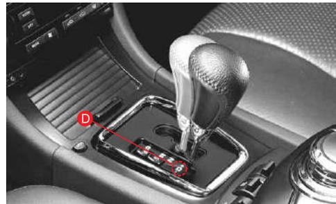
Select this position for normal forward driving on public roads and highways. At this position, the transmission is automatically shifted from the **1st** gear through the **5th** gear according to the vehicle speed.
