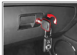
Turn the master key clockwise to unlock the glove box.
