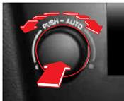
Pressing this switch lights up the **AUTO** indicator on the display. The air flow and air vent will be automatically controlled according to the desired temperature.
