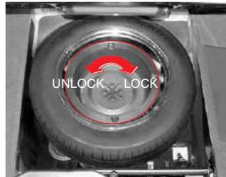
3. Rotate the bowl counter-clockwise and release it.
