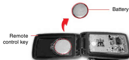
Flip open the rear cover using a suitable tool and replace the battery with new one.
