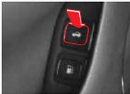
To open the trunk, put the trunk lock switch in the glove box to the unlock position and press this switch.
