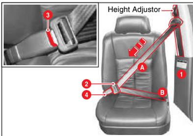
1. Sit back in the seat with the seatback in an upright position and wear the seat belt.
