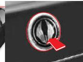
To open the trunk, press and hold this switch when the vehicle is stationary and not in the anti-theft mode.
