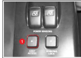
This system is designed to provide the driver sufficient space to access and exit.
