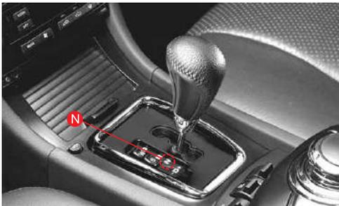
Select this position to stop the vehicle temporarily. At this position, the engine does not transfer power to the wheels and the vehicle will not move. However, for safety, apply the brake while at rest.
