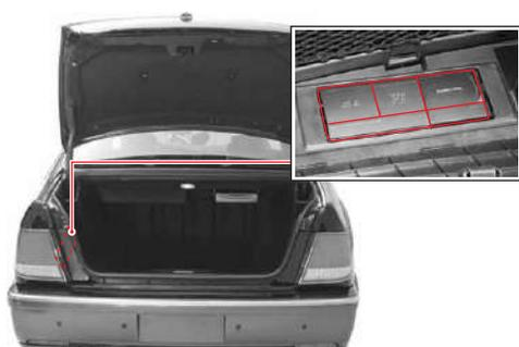
TV tuner and navigation system is installed on the upper part of the trunk. For more information, see separate multi-vision and navigation system manual.
