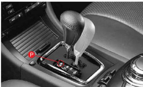
Select this position to park, start the engine, warm-up, and stop the vehicle for a long time.
