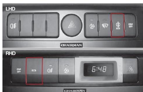
The electronic controlled ECS system minimizes the vertical vibration of the vehicle to enhance driving comforts and steering stability.
