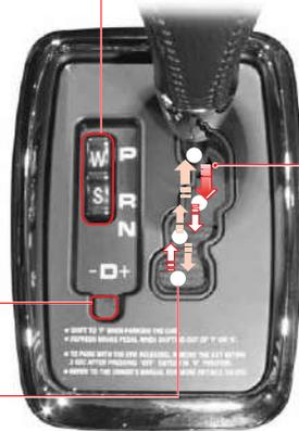
Always apply the brake when shifting from the "P" position with the ignition on.
