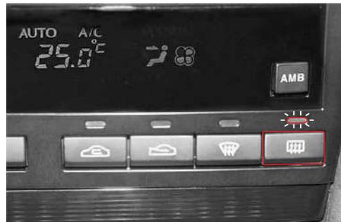
If you press the defogger switch, the integrated heated wire in the rear glass, outside rear view mirror and windshield (RHD model only) operates for 12 minutes then shuts off automatically. When in use, the indicator above the switch comes on.
