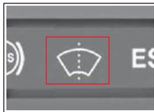
This indicator lights when the washer fluid is low.
