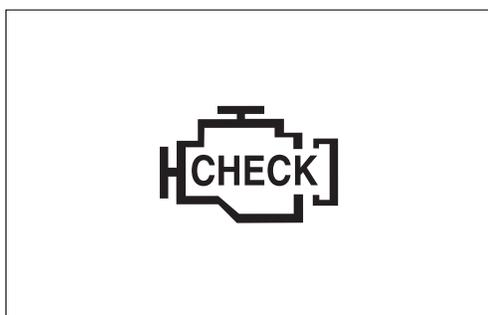
The check engine indicator on the instrument cluster comes on when the fuel or major electronic systems of the engine are not working properly. As a result, the engine's power output may decrease or the engine may stall. If this happens, please visit the nearest Ssangyong dealer or authorized service operator.
