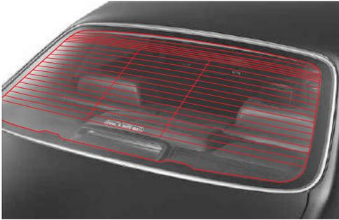
Glass antenna (for FM and AM) is on the upper and lower section of the rear window and the heating grids are on the center section of the rear window.
