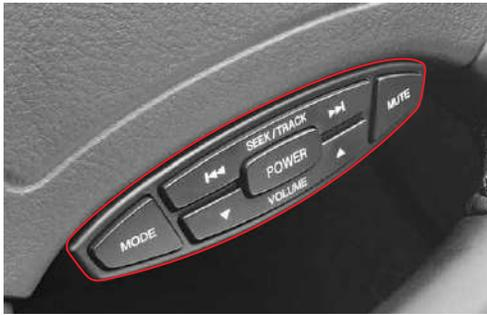
The remote audio control switch is located at the bottom of the steering wheel.
