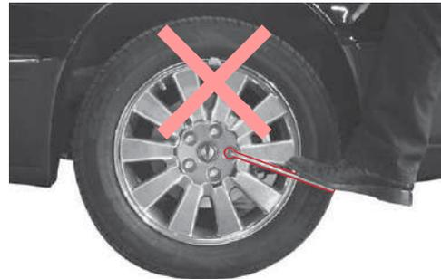
7. Raise the vehicle by rotating the jack connection rod clockwise until the tire is off ground about 3cm.
