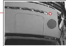
This senses the ambient illumination intensity to determine the timing for turning the headlamp and tail lamp on or off automatically when the light switch is set to "AUTO".
