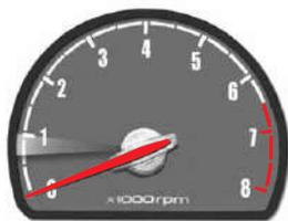
This gauge indicates the engine speed in revolutions per minute. The pointer number multiplied by 1000 is the current engine rpm.
