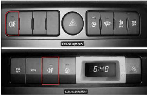
The rear fog light is activated when the tail lamp is on.
