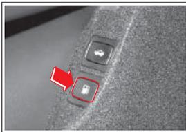
To open the fuel filler lid, push the opening switch at the driver's door trim.
