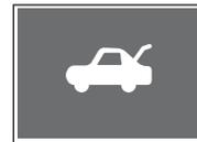
This warning lamp comes on when the trunk is not securely closed.
