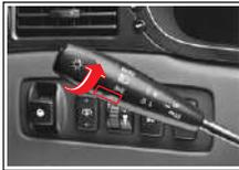
Turn the barrel on the end of the lever as shown, then lights will be operated as follows:
