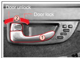
1. Move the driver's door lock button (2) to unlock position (rearward) to unlock the driver's door.
