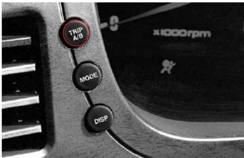
TRIP A/B switch is used for the display mode: TRIP A, TRIP B, and ODO (total driving distance)
