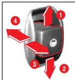
Move the switch until you get the desired position of the steering wheel.
