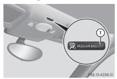
Passenger front air bag off indicator lamp ① illuminates when the passenger front air bag is deactivated.
