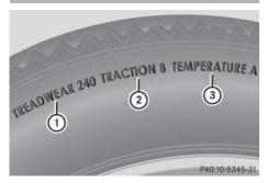
The Uniform Tire Quality Grading is a U.S. Government requirement designed to give drivers consistent and reliable information regarding tire performance. Tire manufacturers are required to grade tires based on three performance factors: tread-
