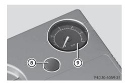
► Check the tire inflation pressure using pressure gauge ⑨.
