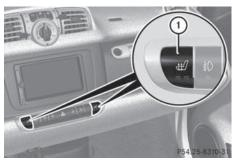
The seat heating has two levels. The indicator lamps on seat heating switch (1) come on to show which heating level you have selected.
