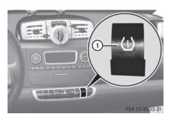
▶ Press Restarting TPMS button ①. The combination low tire pressure/TPMS malfunction telltale in the instrument cluster (▷ page 23) flashes for approximately 5 seconds and then goes out.
