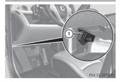
Your vehicle is equipped with a high-voltage disconnect device (1) to disable the vehicle's high-voltage system.
