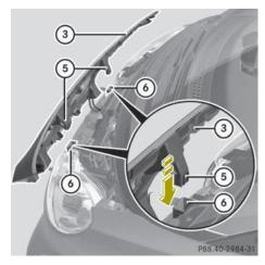
▶ Insert hooks ⑤ on the back of service flap ③ into openings ⑥.
