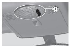
▶ **Removing:** Use a flat object to pry the lamp lens ① off from the passenger side.
