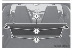
If you wish to use cargo compartment cover blind (1) as normal, assemble it in top mountings (2). If you do not need the cargo compartment cover blind, insert in bottom mountings (3).
