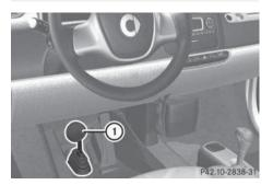
If a brake circuit has failed (▷ page 167), you must depress brake pedal (1) further down to achieve the same effect and the braking distance is increased.
