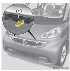
▶ Press both levers ② into the radiator grille until they engage.
