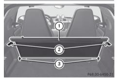
If you wish to use cargo compartment cover blind ① as normal, assemble it in top mountings ②. If you do not need the cargo compartment cover blind, insert in bottom mountings ③.
