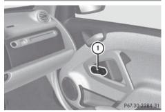
Crank for side window on passenger door
