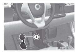
If a brake circuit has failed (▷ page 164), you must depress brake pedal ① further down to achieve the same effect and the braking distance is increased.
