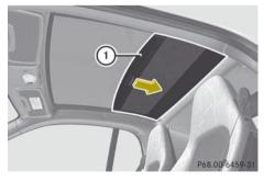
▶ **Opening or closing:** Move sun screen ① forward or backward using the handle.
