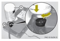
Screw tire sealant container (9) onto flange (10).
