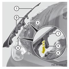
► Insert hooks ⑤ on the back of service flap ① completely into openings ⑥.
