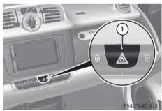
Switching on: Press hazard warning flasher switch (1).
