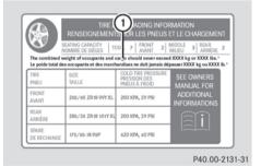
The Tire and Loading Information placard showing load limit information ① is located on the driver's door B-pillar (▷ page 130).
