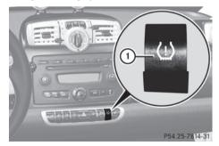
▶ Press Restarting TPMS button ①. The combination low tire pressure/TPMS malfunction telltale in the instrument cluster (▷ page 22) flashes for approximately 5 seconds and then goes out.
