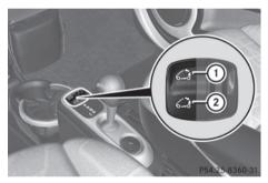
Retractable soft top switch (1) Closing (2) Opening
