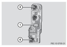
Left bulb carrier with bulb sockets (right bulb carrier in reverse)
