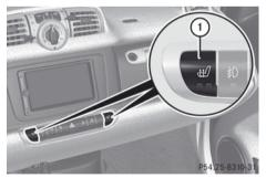
The seat heating has two levels. The indicator lamps on seat heating switch ① come on to show which heating level you have selected.
