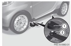
Position jack (2) under take-up bracket (1) so that it is always vertical as seen from the side, even if the vehicle is parked on an incline.
