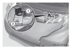
The coolant reservoir is located in the front compartment on the driver's side.
