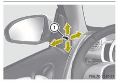
Adjusting: Move adjustment lever ① up, down, left, or right to the desired setting.
