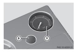
Check the tire inflation pressure using pressure gauge (9).
