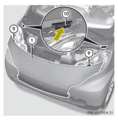
► Insert both tabs ③ on the back of service flap ① completely into openings ⑩.
