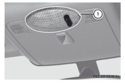
▶ **Removing:** Use a flat object to pry the lamp lens ① off from the passenger side.
