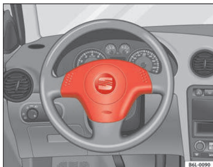
Fig. 17 Driver airbag located in steering wheel
