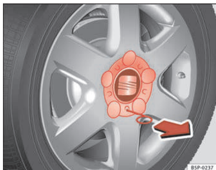
Fig. 131 Changing the wheel: Removing a hub cap
