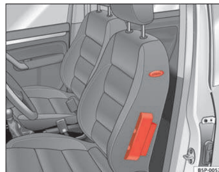
Fig. 21 Side airbag in driver seat
