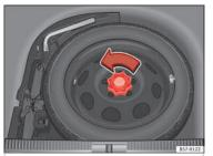
Fig. 230 Compact temporary spare wheel: raised floor panel.
