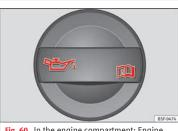
Fig. 60 In the engine compartment: Engine oil filler cap
