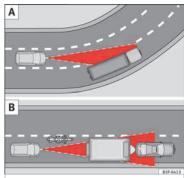
Fig. 184 (A) Vehicle on a bend. (B) Motorcyclist ahead out of range of the radar sensor.
