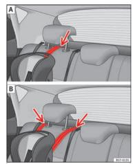
Fig. 33 Retainer strap: adjustment and assembly according to the Top Tether belt.
