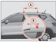
**Fig. 162** Attachment points for the roof railings for the roof carrier system.
