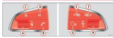
Fig. 120 Controls on the steering wheel.
