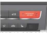
Fig. 51 Warning lamp for disabling the front passenger airbag.
