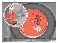
Fig. 231 In the luggage compartment: remove the subwoofer.
