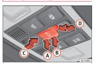
Fig. 134 On the interior roof lining: sunroof button.
