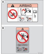
Fig. 28 Airbag stickers - version 1: on the front passenger's sun visor  $\boxed{\mathbb{A}}$  and on the rear frame of the front passenger's door  $\boxed{\mathbb{B}}$ .
