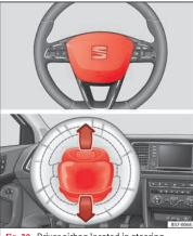
Driver airbag located in steering Fig. 20 wheel.
