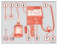
**Fig. 96** Standard representation: contents of the anti-puncture kit.
