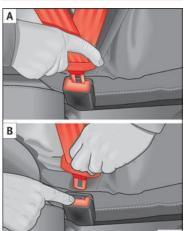
Fig. 16 Positioning and removing the seat belt buckle.
