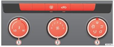
Fig. 57 In the centre console: heating system and fresh air controls.
