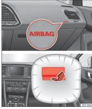
Fig. 21 Front passenger airbag located in dash panel.
