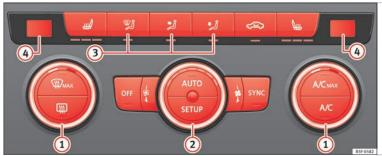
Fig. 55 In the centre console: Climatronic controls
