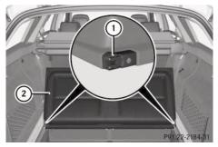
➤ To remove: fold seat cushion ② upwards and remove it from seat cushion guides ①.
