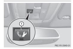
▶ Press and hold Roadside Assistance button ① for more than two seconds.
