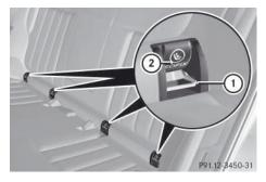
When installing the LATCH-type (ISOFIX) child restraint system, fold protective caps ② of securing rings ① inwards.
