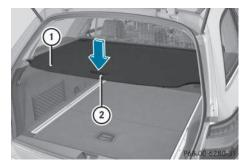
► To retract: unhook cargo compartment cover ① from the retainers on the left and right and guide it forwards by grab handle ② until it is fully retracted.
