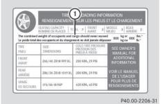
► Specification for maximum permissible load ① is listed on the Tire and Loading Information placard: "The gross weight of occupants and luggage must not exceed XXX kg or XXX lbs."
