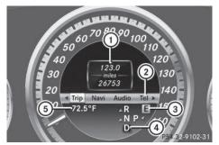
Example: multifunction display for DIRECT SELECT automatic transmission
