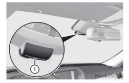
▶ Fold down the camera cover by recess (1).
