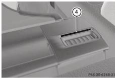
Make sure that red lock status indicator ④ is no longer visible. The combined cargo cover and net will otherwise not be locked in place.
