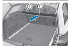
➤ To extend: pull cargo compartment cover ① back by grab handle ② and clip it into the retainers on the left and right.
