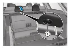
▶ Press release button ① and fold the head restraints down.
