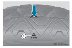
Bar marking (1) for tread wear is integrated into the tire tread.
