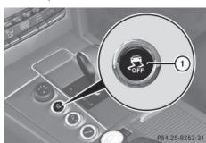
► To deactivate: press button ① until the ESP® OFF warning lamp lights up in the instrument cluster. The ☐ OFF message appears in the
