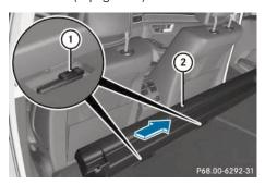
► Insert combined cargo cover and net ② into the two guides ① and push it up to the stop in the direction of the arrow.
