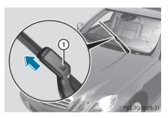
► Firmly press release knob ① and pull the wiper blade upwards from the wiper arm in the direction of the arrow.
