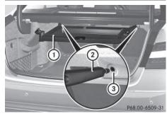
► To install: insert retainer ② of box ① into slots ③
