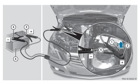
Position number (6) identifies the charged battery of the other vehicle or an equivalent jump-starting device.
