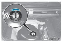
► Turn DEF cap ① counter-clockwise and remove it.
