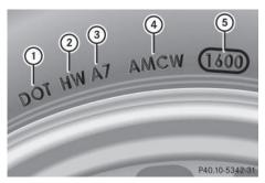
The TIN is a unique identification number. The TIN enables the tire manufacturers to inform purchasers of recalls and other safety-relevant matters. It makes it possible for the purchaser to easily identify the affected tires. The TIN is made up of manufacturer identification code ②, tire size ③, tire type code ④ and manufacturing date ⑤.
