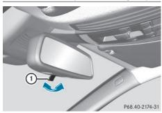
➤ anti-glare mode: flick anti-glare switch ① forwards or back.
