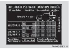
Example: tire pressure table with tire dimensions Some tire pressure tables show only the rim diameters instead of the full tire size, e.g. **R18**. The rim diameter is part of the tire size and can be found on the tire sidewall (> page 364).
