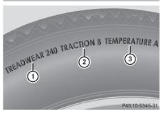
Uniform Tire Quality Grading Standards are U.S. government specifications. Their purpose is to provide drivers with uniform reliable information on tire performance data. Tire manufacturers have to grade tires using three performance factors: tread wear (1), tire traction (2), and heat resistance (3). All tires sold in North America are provided with the corresponding quality class mark on the sidewall of the tire, even though these regulations do not apply to Canada.
