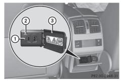
115 V socket ① provides an alternating voltage of 115 V, so that small electronic devices can be connected. These devices, such as game consoles, chargers and laptops, together should not consume more than a maximum of 150 W.
