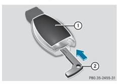
▶ Press mechanical key ② into the opening in the SmartKey in the direction of the arrow until battery tray cover ① opens. When doing so, do not hold cover ① shut.
