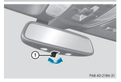
► anti-glare mode: flick anti-glare switch (1) forwards or back.
