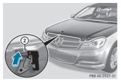
Reach into the gap, pull hood catch handle (2) up and lift the hood.
