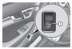
► **To open:** pull remote operating switch for trunk lid ① until the trunk lid opens.
