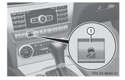
▶ To deactivate: press button (1) until the ESP<sup>®</sup> OFF warning lamp lights up in the instrument cluster.
