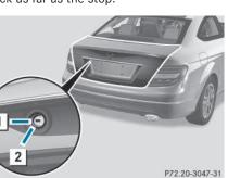
Turn the mechanical key counter-clockwise from position 1 as far as it will go to position 2.
