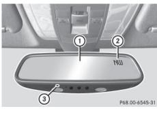
To obtain a correct display in rear-view mirror (1), the compass must be calibrated and the magnetic field zone must be set.
