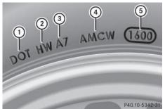
The TIN is a unique identification number. The TIN enables the tire manufacturers to inform purchasers of recalls and other safetyrelevant matters. It makes it possible for the purchaser to easily identify the affected tires. The TIN is made up of manufacturer identification code (2), tire size (3), tire type code (4) and manufacturing date (5).
