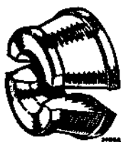
18G 264 E and 18G 264 F. Bevel Pinion Bearing Outer Race Remover Adaptors—Rear.
