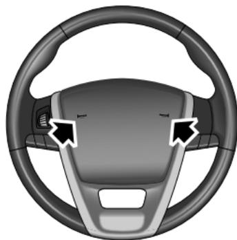
When the ignition switch is in position I or II, press the steering wheel pad where arrowed to operate the horn.
