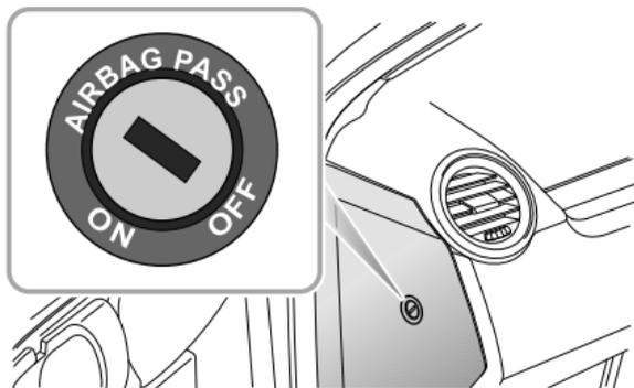
The airbag disable switch is located on the end of the dashboard. To disable the passenger airbag, insert the emergency key blade contained within the handset. To remove the emergency key from the handset refer to the Starting and Driving Emergency Unlocking section of the owners handbook.
