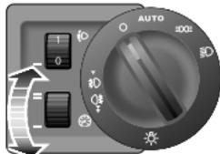
When the ignition is in position II, and the sidelamps or dipped headlamps are on, rotate the control up to increase or down to decrease instrument illumination. The instrument dimmer also controls the backlight illumination of switches, audio system, message centre and the satellite navigation system (if fitted). When the sidelights are switched on the message centre display on the instrument pack and the satellite navigation system (if fitted) will dim automatically.
