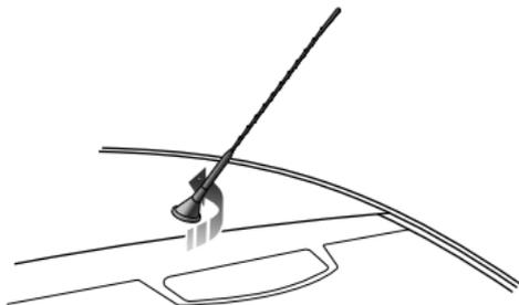
The antenna is located at the rear of the roof. Avoid bending the antenna. However when required, e.g. when using an automatic car washing facility, please ensure that the antenna is removed.
