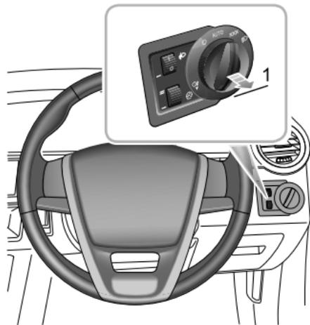
*Note: The rear fog lights are switched off automatically when the main lighting switch is turned off.*
