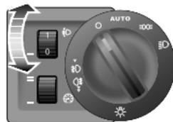
The angle of the dipped beam is affected by the distribution of passenger and luggage weight within the car.
