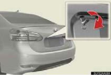
Turn the mechanical key clockwise to open.
