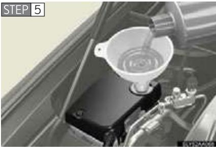
Add engine coolant if necessary.
