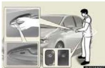
Touch both lock sensors on the upper and lower part of the door handle simultaneously.
