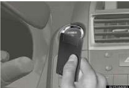
**STEP 3** To change “POWER” switch modes: Within 10 seconds of the buzzer sounding, release the brake pedal and press the “POWER” switch. Modes can be changed each time the switch is pressed. (→P. 148)
