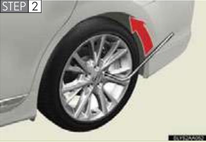
Slightly loosen the wheel nuts (one turn).
