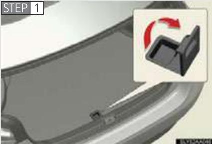
Lift up the hook and remove the panel.
