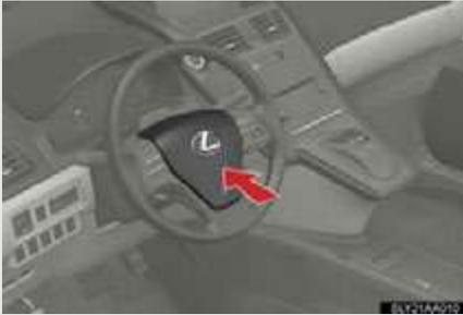
To sound the horn, press on or close to the
