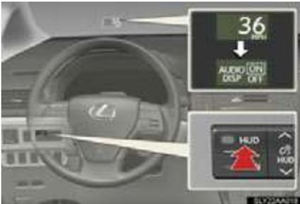
With the touch tracer display ON/OFF selection mode displayed, press and hold HUD (Head-up Display) main switch for more than 2 seconds again to enter audio display ON/OFF selection mode. ON or OFF can be selected by pressing HUD (Head-up Display) main switch.
