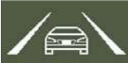
Displays a warning message that alerts the driver of a deviation from the lane through use of the lane departure warning function. (→P. 511)
