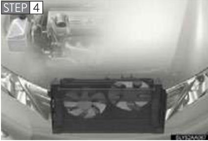
After the hybrid system has cooled down sufficiently, check the engine coolant level and inspect the cooling system for leaks.
