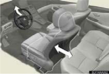
Exiting the vehicle: When all of the following actions have been performed, the steering wheel will move up and back to the point farthest away from the driver and the seat will move backward (auto away function):
