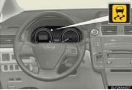
If the vehicle is in danger of slipping or if any of the drive wheels spins, the slip indicator light flashes to indicate that the VSC/TRAC systems are operating.
