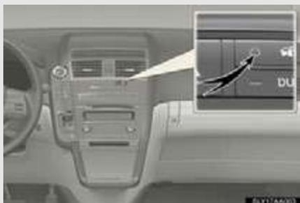
Close the doors, trunk and hood, and lock all the doors using the entry function or wireless remote control. The system will be set automatically after 30 seconds.
