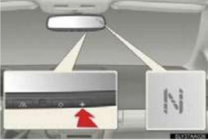
To turn the compass on or off, press the button for more than 3 seconds.
