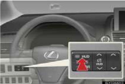
Pressing the switch turns the head-up display on/off and changes the vehicle speed display units as follows:
