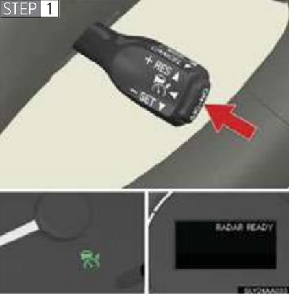
Press the “ON-OFF” button to activate the cruise control.
