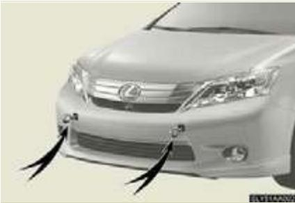
If a tow truck is not available in an emergency, your vehicle may be temporarily towed using a cable or chain secured to the emergency towing eyelet(s). This should only be attempted on hard surfaced roads for short distances at under 18 mph (30 km/h).
