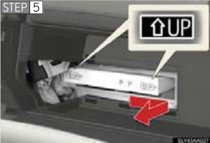
Slide and pull out the filter. Replace the filter with a new one.
