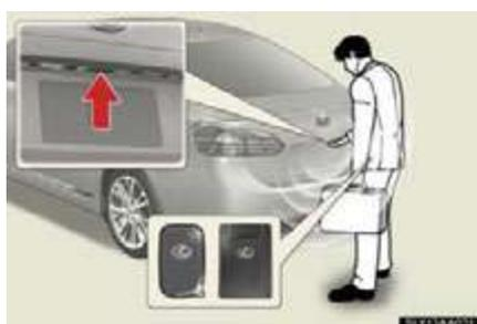
Press the button to unlock the trunk.
