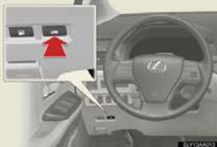
Press the opener switch to release the trunk lid.
