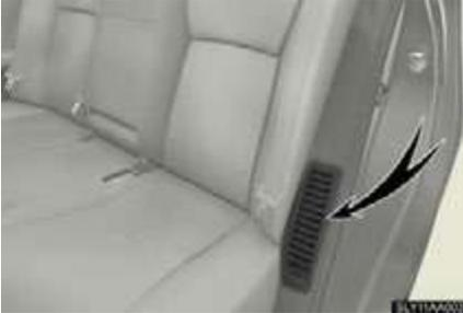
There is an air intake vent on the side of the rear left seatback for the purpose of cooling the hybrid battery (traction battery). If the vent become blocked, the hybrid battery may overheat, leading to a reduction in hybrid battery output.
