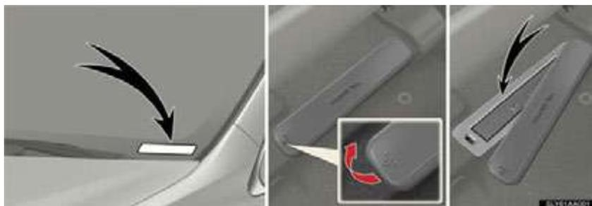
This number is stamped on the top left of the instrument panel and under the front passenger's seat (on some models).
