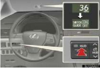
Pressing and holding the HUD (Head-up Display) main switch for more than 2 seconds changes the display to touch tracer display ON/OFF mode. Press the HUD (Head-up Display) main switch to select ON or OFF.
