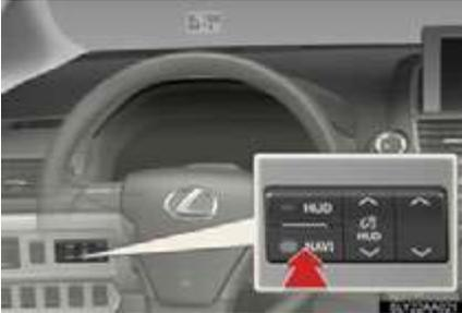
Pressing the switch turns the turn-by-turn navigation on/off, when the head-up display is on.
