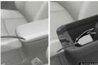
When the console box is open, portable audio device cables can be pulled through the opening.
