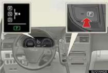
Fully stop the vehicle and keep depressing the brake pedal, and then press the P position switch.
