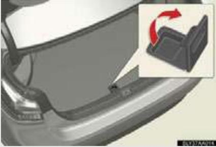
Pull the lever upward to lift up the luggage mat.
