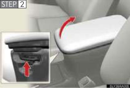
Pull up the knob to release the lock and lift the armrest.
