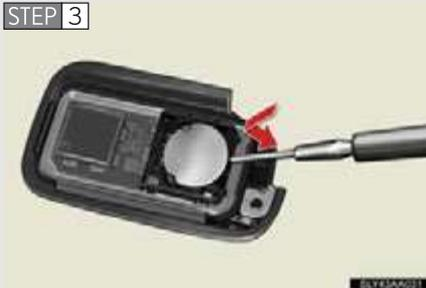
Remove the depleted battery.
