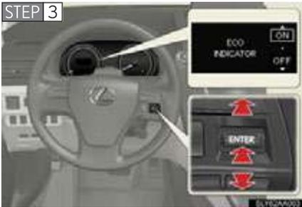
Press the “ENTER” switch upwards or downwards to select the desired setting for the item being customized and press the “ENTER” switch to confirm.
