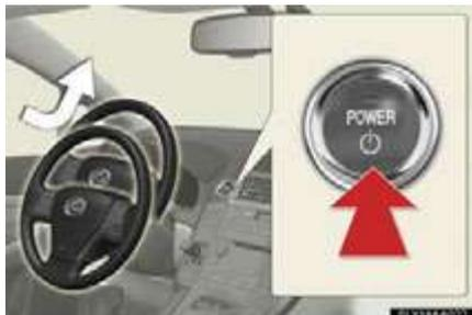
When the “POWER” switch is turned off, the steering wheel returns to its stowed position by moving up and away to enable easier driver entry and exit.
