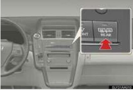
Turns the rear window and outside rear view mirror defoggers on/off
