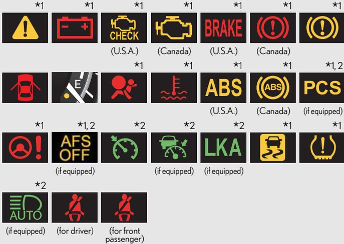
\*1: These lights turn on when the “POWER” switch is turned to ON mode to indicate that a system check is being performed. They will turn off after the hybrid system is on, or after a few seconds. There may be a malfunction in a system if a light does not turn on, or if the lights do not turn off. Have the vehicle inspected by your Lexus dealer.
