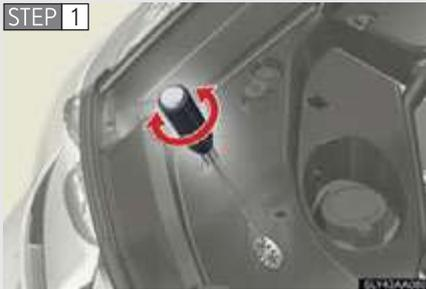
Using a Phillips-head screwdriver, turn bolt A in either direction.
