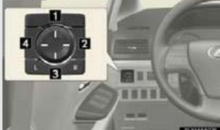
To adjust the mirror, press the switch.
