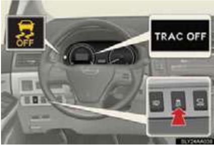
To turn the TRAC and VSC systems off, press and hold the button for more than 3 seconds while the vehicle is stopped.
