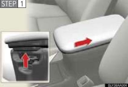
Pull up the knob to release the lock and slide the armrest.
