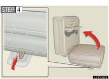
Unlock the seat legs by pulling the seat leg lock release handles, and lift the seats sideward.
