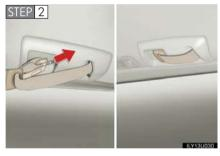
Stow the seat belt tabs in the cover set in the roof as shown.
