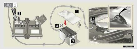
Connecting the jumper cables.
