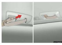
For the center seat belt, stow the seat belt tabs in the cover set in the roof as shown.
