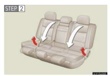
Fold down the seatbacks while pulling the lock release levers.
