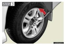
Slightly loosen the wheel nuts (one turn).
