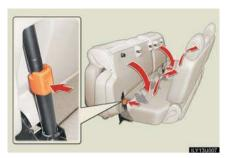
Push the red knobs and swing the seat down, then raise the seat-backs.
