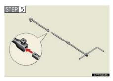
Attach the hooked jack handle end to the jack handle extension as shown.
