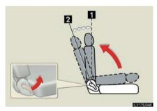
Fold the seatback forward and then back to the 1st lock position (most upright position) until it locks into place. Adjust the seatback to the 5th lock position.
