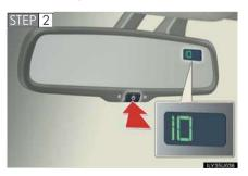
Press the button until a number (1 to 15) appears on the compass display.
