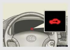
To arm the alarm, exit the vehicle, make sure that the doors and hood are closed, and lock all the doors.
