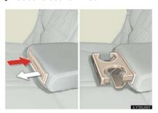
To open, press in and release the rear cup holder on the armrest.
