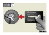
Bring the key case close to the engine switch within 10 seconds as indicated by an arrow.
