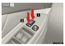
Shift the shift lever to "P" or "N", press and hold the driver's door lock switch (11 or 22) for 5 seconds then release.
