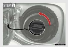
To remove the fuel tank cap, turn the cap slowly counterclockwise, then pause slightly before removing it.
