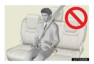
Do not use the third center seat belt with either buckle released. Fastening only one of the buckles may result in death or serious injury in case of sudden braking or a collision.
