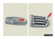
An insulating sheet is set to prevent the batteries from being discharged. Remove the insulating sheet before using the remote control.
