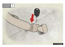
To release the hooked tab, insert the vehicle's key into the hole on the buckle with the light gray buckle release button.
