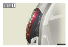
Open the back door and remove the screws.
