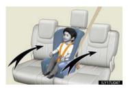
When installing a child restraint system in the third center position, set the both seatbacks to the same angle. Otherwise, the child restraint system cannot be properly secured
