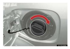
When installing the cap, turn it clockwise until one click is heard, in order to fully close it.
