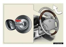
When the ignition key is removed, the steering wheel returns to its stowed position by moving up and away to enable easier driver entry and exit
