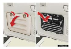
Remove the tool tray compartment cover and take out the tool tray.
