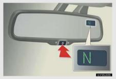
Press the button to turn the compass on/off.
