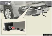
Insert the jack handle extension into the lowering socket.
