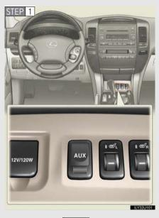
Connect the portable audio device.
