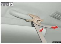
Pull the free end of the straps to the secure the seats.
