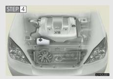
After the engine has cooled down sufficiently, check the coolant level and inspect the radiator for any leaks.
