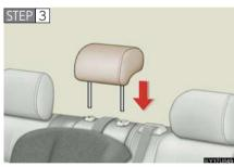
Reinstall the head restraint.
