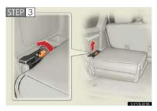
Remove the seat lock cover and push the red seat lock release knobs outward, then lift the seats free.
