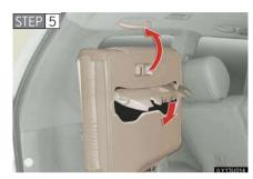
Retract the seat legs, then take the holding straps out and attach the straps to the assist grips.
