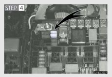
Remove the fuse with the pullout tool.
