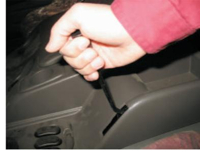
Tractor adopts separate trailer brake hand brake valve, its function is: auxiliary brake the trailer by controlling separately, especially for complete train running on ramp to lighten impulsion from trailer and make train decelerate calmly as well as increasing stabilization when braking.
