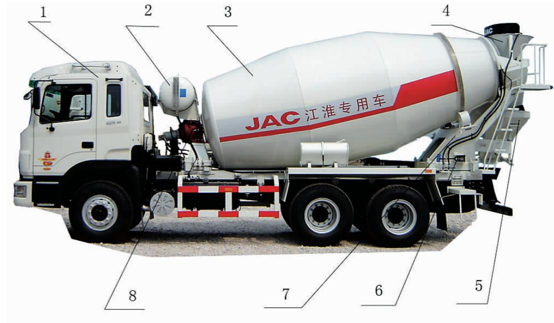
1. 2nd category chassis; 2. water supply system; 3. agitating tank; 4. feed system; 5. output system; 6. operation system; 7. frame system; 8. hydraulic drive system
