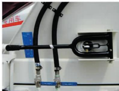
b. The agitating of the pre-agitating concrete and agitating truck: must pull the handle to "agitating" position during driving when the agitating truck is fully loaded with concrete;
