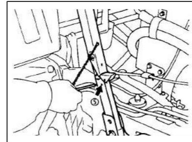
5. Push the cab all the way up, and the cab will be automatically held in position by the cab stay. Insert the safety pin (5).
