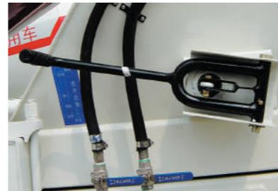
c. Stuff output of pre-agitating concrete: pull the operation handle to "low speed" or "high speed" position, meanwhile lock the stuff collecting trough in a specific position.
