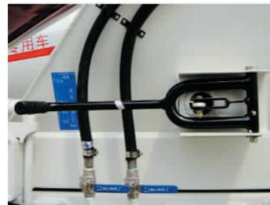
d. The stop of the agitating tank: pull the operation handle to "stop".
