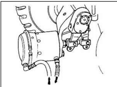
8. Measure the stroke made by the push rod of the brake chamber when the brake pedal is depressed all the way. Verify that the stroke is up to specifications given in the following table if it is out of specification, adjust with the worm shaft.
