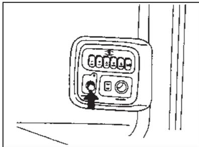
**BED TEMPERATURE ADJUSTABLE KNOB (If installed)**
