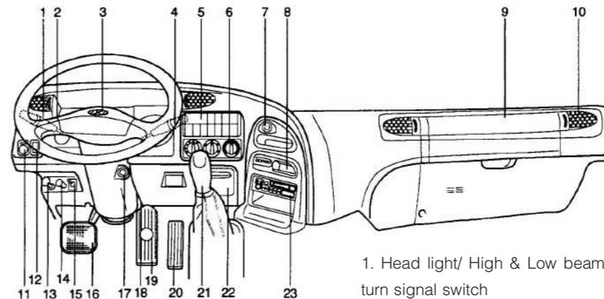
1. Head light/ High & Low beam/ turn signal switch
