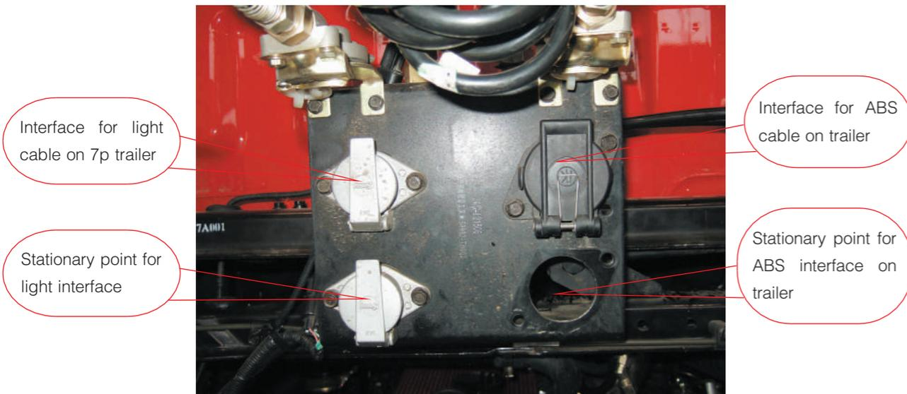
Trailer cable device includes trailer light cable assembly and trailer ABS assembly. Cable is fixed on plug, and trailer light cable is used to control light and signal on trailer.
