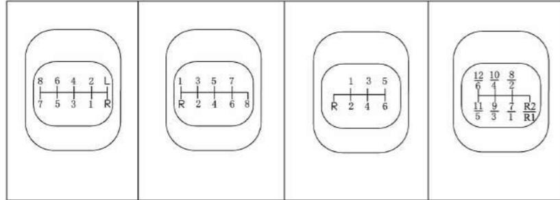
Your Manual Transmission vehicle has a fully synchro-meshed, 8-forward and 1-reverse or 5-forward and 1-reverse speed transmission controlled by a gear shift, lever located on the floor. This shift pattern is shown on the knob.
