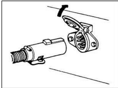
Connect the air hoses and open the air service valve. Then, push the cab control valve in and supply air to the trailer.
