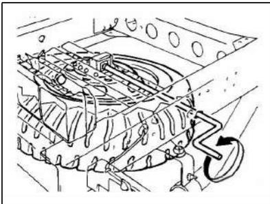
2. To install a tire, face the convex side of wheel upward, put the hanging plate in the disc wheel, and rotate the spare tire carrier handle clockwise to lift the tire.
