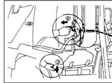
3. Hold the grip (3) of the cab. While pressing it down, pull the safety hook (4).
