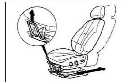
**Adjusting Seat Forward and Rearward (If installed)(Driver's side only)**
