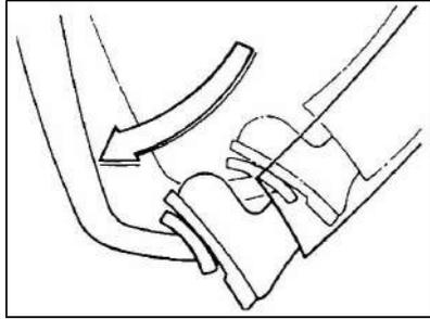
2. Remove the rubber cap from the air bleeder of the clutch booster, mount one end of a transparent vinyl hose, and put the other end in a bowl containing brake fluid.
