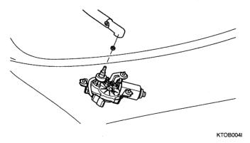
Tightening torque 14-17 Nm (140-170 kg·cm, 10.3-12.5 lb·ft)
