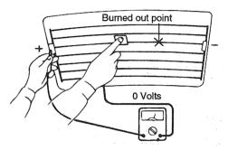
To check for open circuits, slowly move the test lead in the direction that the open circuit seems to exist. Try to find a point where a voltage is generated or changes to 0V. The point where the voltage has changed is the open-circuit point.
