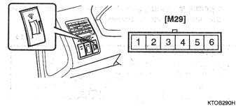
Check for intensity. If the light intensity of the lamps changes smoothly without any flickering when the rheostat is turned, it can be assumed that the rheostat is normal.
