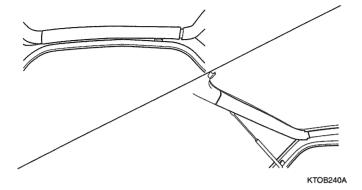
Remove the tailgate trim panel after removing 4 screws.
