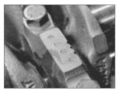
7C.69 Identification notches on No. 3 main bearing cap
