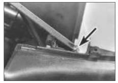
21.3 Removing instrument panel screw
