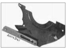
Fig. 1.20 Flywheel housing cover plate removed (Sec 13)
