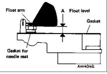
Fig. 3.16 Float setting diagram (Solex C32 DISA 11) (Sec 10)
