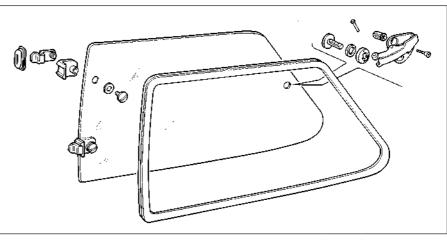
Fig. 12.18 Components of opening side window (Sec 18)
