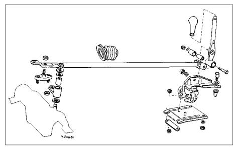
Fig. 13.92 Exploded view of the gear selector and control road assembly components fitted to 1372 cc models (Sec 12)
