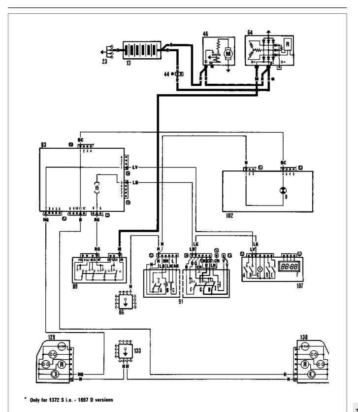
Wiring diagram 37 - rear foglamps (1990-on 45 and 55 models)
