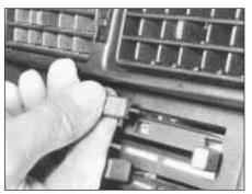
12.5 Pulling off heater control lever knob
