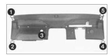
Fig. 12.20 Rear view of facia panel showing fixing screw locations (Sec 22) 2, 3 and 4 Screws 1 and 5 Clips
