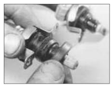
9C.95A Fuel injector large seal
