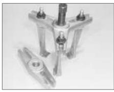
Three-legged hub and bearing puller
