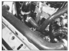
9C.55D Air cleaner metal duct over radiator
