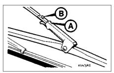
Fig. 9.7 Tailgate wiper blade fixing (Sec 26) A Hole B Peg
