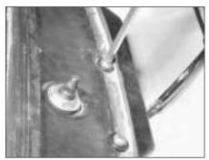
25.4 Removing windscreen wiper motor mounting screws
