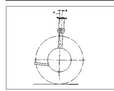
Fig. 10.7Castor angle (Sec 8)AVertical lineBCastor angle (positive)
