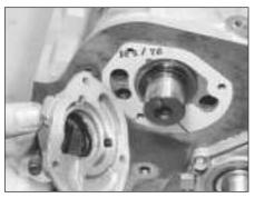
42.10A Auxiliary shaft end plate and gasket
