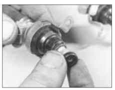
9C.95B Fuel injector small seal
