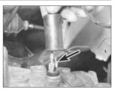
44.22A Reversing lamp switch on transmission
