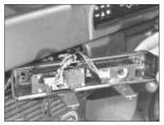
15.63 . . . and withdraw the auxiliary control panel
