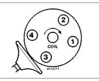
Fig. 4.15 Spark plug connections on 1116 cc and 1301 cc engines (Sec 11)
