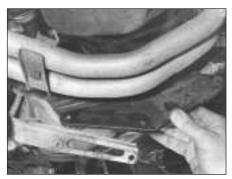
5B.61 Removing the flywheel housing cover plate
