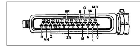
Fig. 13.80 Microplex ignition system ECU multipin connector (Sec 10) For colour code, see main wiring diagrams
