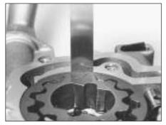
5B.74A Checking the oil pump gear-tohousing clearance
