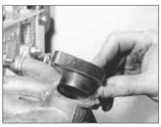
9B.19 Carburettor insulator block
