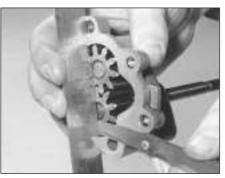
7B.177 Checking the gear endfloat
