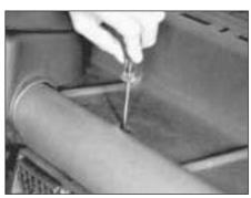
Fig. 2.8 Extracting heater upper fixing screw (Sec 12)
