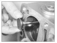
17.17B Inserting a valve into its guide
