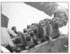
7D.10 Lower the crankshaft into position
