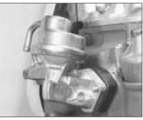
3.6A Fuel pump on mounting studs
