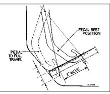
Fig. 13.87 Clutch pedal adjustment diagram - cable clutch (Sec 11)
