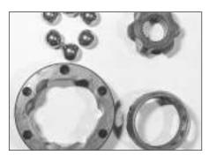
13.19C Components of CV joint
