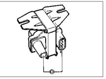
Fig. 13.84 Test connections for ignition coil secondary windings check - Digiplex 2 ignition system (Sec 10)
