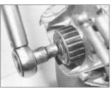
5D.16B Tightening the crankshaft sprocket bolt
