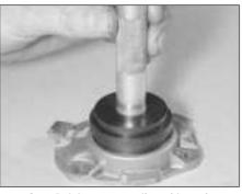
7C.53 Driving a new oil seal into the auxiliary shaft cover
