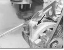
4.2B Alternator adjuster bolt
