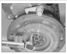
7B.158B . . . tighten the bolts to the specified torque
