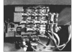
15.26A Fuse block on the 1301 cc Turbo ie model
