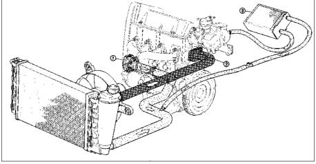
Fig. 13.26 Cooling system circuit - 999 and 1108 cc engines (Sec 8A) 1 Coolant pump 2 Thermostat 3 Heater matrix
