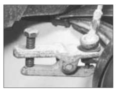
2.2 Disconnecting a tie-rod end balljoint
