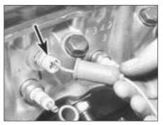
44.26B Coolant temperature switch
