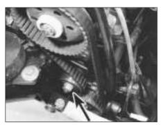
6B.20 Belt tensioner pulley locknut (arrowed)
