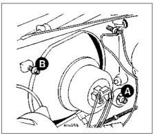
Fig. 9.3 Headlamp beam adjustment screws (Sec 17) A Vertical B Horizontal
