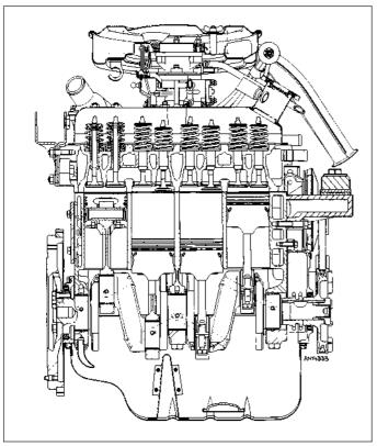
Fig. 1.1 Longitudinal section of 903 cc engine (Sec 1)
