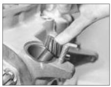
42.15 Fitting oil pump driveshaft
