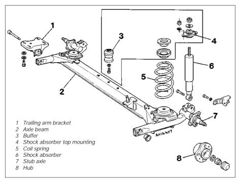
Fig. 11.8 Rear suspension components (Sec 8)
