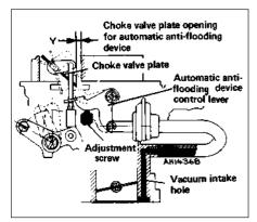
Fig. 3.27 Anti-flooding device (automatic) adjustment diagram (Weber 30/32 DMTR 90/250) (Sec 14)
