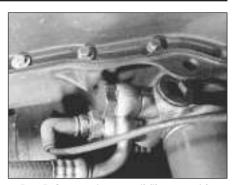
6B.24B Connections at oil filter cartridge mounting base
