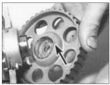
5B.22C Camshaft sprocket showing integral key (arrowed)
