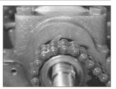
6.13C Self-tensioning links on inside of chain
