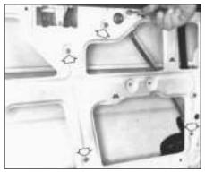
Fig. 12.9 Door window regulator fixing screws (Sec 12)
