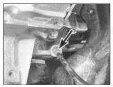
23.3 Speedometer cable connector at transmission
