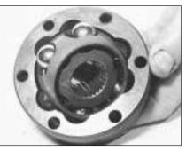
13.18 Removing inboard CV joint ball/cage assembly from outer track
