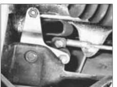
12B.31 Gear control and selector link rod joints
