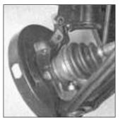
Fig. 1.18 Hub carrier detached from strut clamp (Sec 13)
