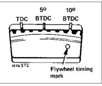
Fig. 4.5 Flywheel housing timing marks (Sec 4)
