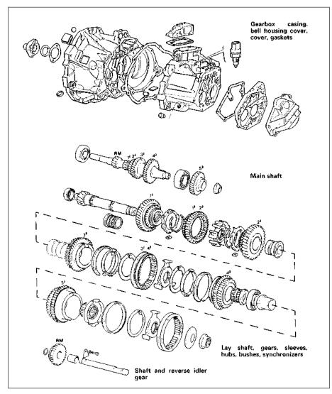
Fig. 13.90 Exploded view of the transmission unit fitted to 1372 cc models (Sec 12)
