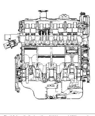
Fig. 1.3 Longitudinal section of 1116 cc and 1301 cc engines (Sec 1)
