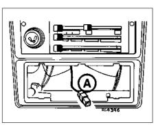
Fig. 9.8 Radio housing and power lead (A) (Sec 30)
