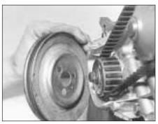
5D.22 Crankshaft pulley installation
