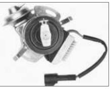
Fig. 13.72 Rotor aligned with arrow on distributor dust shield - 999 and 1108 cc engines (Sec 10)
