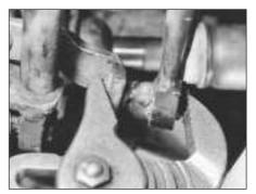
5D.45 Connecting ball socket type gearchange rod
