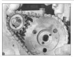
6.13A Fitting the sprockets and timing chain
