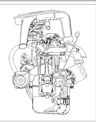
Fig. 1.2 Cross-section of 903 cc engine (Sec 1)
