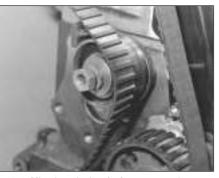
28.8 Slipping timing belt onto tensioner pulley
