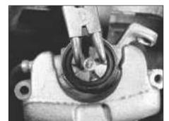
14B.28 Rotating a rear caliper piston
