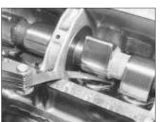
25.4 Checking a valve clearance
