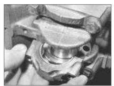
5B.98 Fitting a big-end bearing cap
