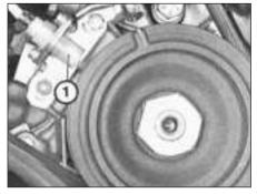
Fig. 13.77 Crankshaft pulley timing mark aligned with timing pointer - Microplex ignition system (Sec 10) 1 TDC sensor
