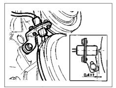
Fig. 4.11 TDC sensor gap (Sec 10)
