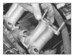
9C.74 Removing an inlet manifold twin pipe stub
