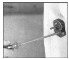
Fig. 12.14 Removing door lock fixing screw (Sec 12)
