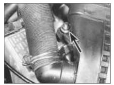
9A.9B Circular type air cleaner nut on the camshaft cover (arrowed)
