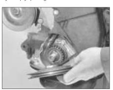
7B.35 Crankshaft pulley removal
