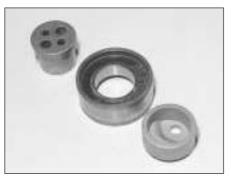
7B.38B The three sections of the timing belt tensioner
