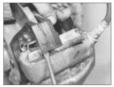
3.2B Removing a locking block
