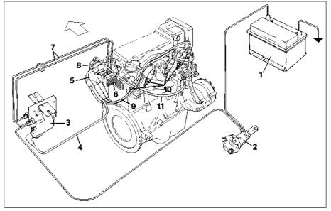
Fig. 13.70 Breakerless ignition system - 999 and 1108 cc engines (Sec 10)
