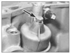
42.16B Crankcase breather and retaining bolt
