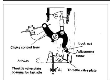
Fig. 3.12 Fast idle adjustment diagram (Weber 32 ICEV 50/250) (Sec 9)
