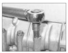
27.18 Tightening a camshaft carrier bolt
