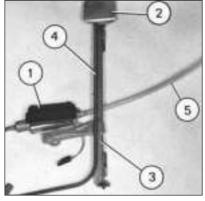
Fig. 9.12 Power operated window components (Sec 31)
