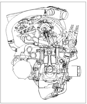
Fig. 1.4 Cross-section of 1116 cc and 1301 cc engines (Sec 1)
