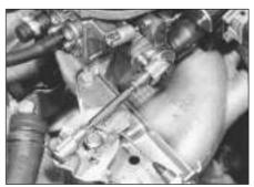
9D.22 Accelerator control rod and cable connections
