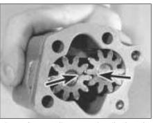
7B.175 Correct alignment of scribed marks (arrowed) on gears
