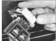
17.34B Disconnecting an electric window regulator switch plug
