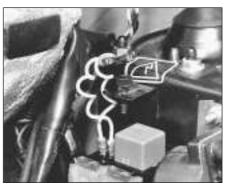
9D.30 Test lead connected to relay terminals 30 and 87
