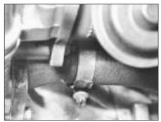
5C.7B Radiator hose at thermostat housing
