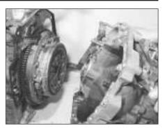
5C.39 Separating the engine and transmission
