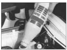
8B.4 Topping up the expansion tank with antifreeze on the 1301 cc engine
