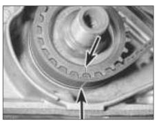
7B.52B Timing belt mark aligned with scribed mark on crankshaft sprocket (arrowed)
