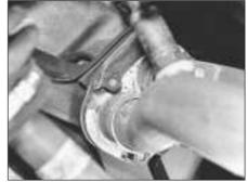
9D.71 Exhaust downpipe to manifold flange connection showing retaining nuts and locktabs
