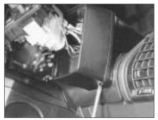
15.55A Facia switch housing lower screw removal on the 1301 cc Turbo ie model
