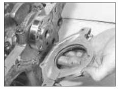
5D.9 Fitting crankshaft rear oil seal retainer
