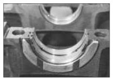
5D.3 Crankshaft thrust washer at centre bearing
