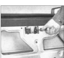
Fig. 12.6 Door glass mounting screw (Sec 12)
