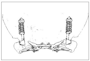
Fig. 11.1 Front suspension arrangement (Sec 1)
