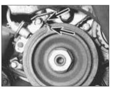
10.39 Crankshaft pulley timing marks (arrowed)
