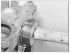
5B.97 Fitting a piston/connecting rod
