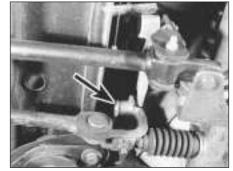
12A.6 Gearchange link rod spring clip (arrowed) on the 1301 cc Turbo ie engine
