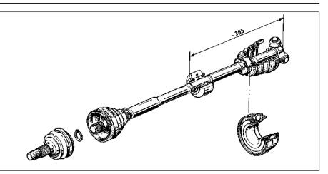
Fig. 13.101 Correct position of driveshaft damper weight on 1108 cc and 1372 cc ie models (Sec 13)
