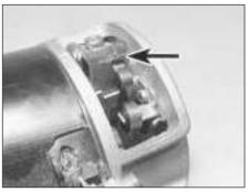
9.4 Starter motor brush partly withdrawn
