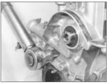
5D.12B Tightening an oil pump bolt
