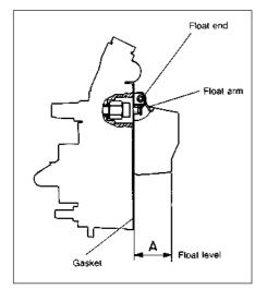
Fig. 13.36 Float level measurement -Weber 32 TLF carburettor (Sec 9B) *A* = 26.75 to 27.25 mm (1.05 to 1.07 in)
