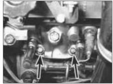
6B.13 Two of the four additional cylinder head bolts (arrowed)
