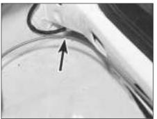
17.15 Tailgate release cable (arrowed)
