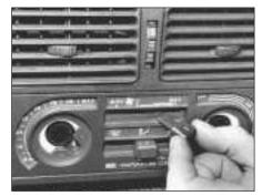
15.68 Remove the control knobs . . .
