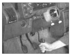
Fig. 10.2 Removing steering column shroud screws (Sec 5)
