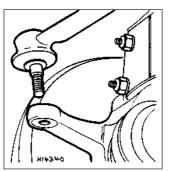
Fig. 1.17 Tie-rod end balljoint disconnected (Sec 13)
