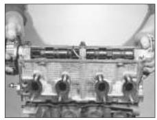
5B.51 Fitting the cylinder head
