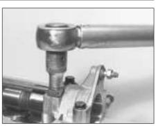
5B.23B Unscrewing the camshaft bearing/banjo union bolt
