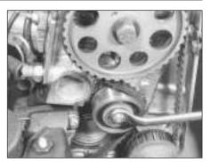
5B.9 Releasing the timing belt tensioner nut
