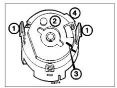
Fig. 4.16 Typical ignition switch (Sec 12)1 Retaining tabs3 Alignment notches2 Switch cam4 Locating projection
