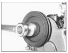
20.23 Tightening crankshaft pulley nut
