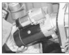
8.3 Removing starter motor
