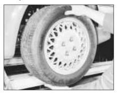
□ If excess free play is suspected at a component pivot point, this can be confirmed by using a large screwdriver or similar tool and levering between the mounting and the component attachment. This will confirm whether the wear is in the pivot bush, its retaining bolt, or in the mounting itself (the bolt holes can often become elongated).
