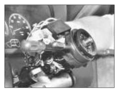
15.47B . . . and remove the column switch
