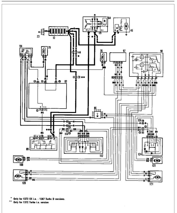
Wiring diagram 49 - electric windows and central locking (1990-on 3-door models)
