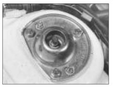
3.4A Strut reinforcement plate
