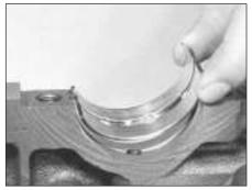
20.1 Fitting a main bearing shell
