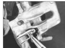
14B.36 Disconnecting the handbrake cable from the caliper lever
