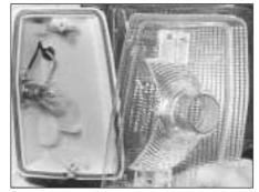
19.4 Front direction indicator lamp lens and bulb
