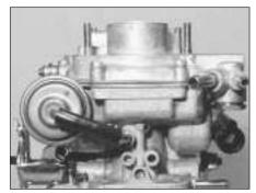
9B.34B Weber 30/32 DMTE carburettor from diaphragm hose side
