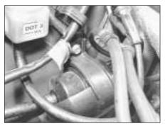
9D.15 Secondary fuel filter element
