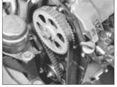
7B.52A Timing belt refitted over the sprockets and tensioner
