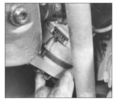
15.4 Removing the alternator from the 999 cc engine
