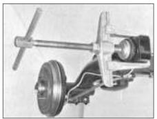
Fig. 11.10 Method of renewing trailing arm bush (Sec 10)
