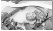
$\Box$  The fluid reservoir must be secure and the fluid level must be between the upper (A) and lower (B) markings.
