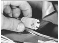
15.59B . . . and disconnect the speedometer cable
