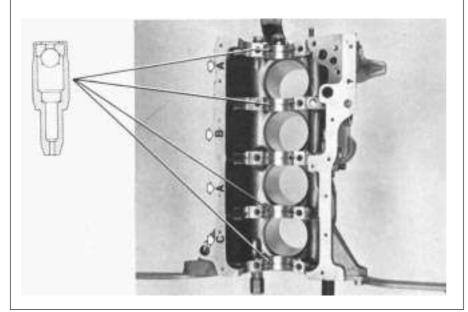
Fig. 13.12 Piston oil spray nozzle locations - 1301 cc Turbo ie engine (Sec 6A) Letters denote cylinder bore grade
