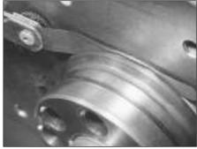
7C.70 Measuring crankshaft endfloat using feeler gauge method
