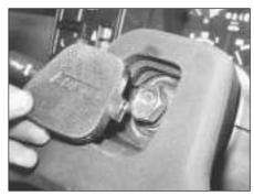
4.2 Removing steering wheel hub plate
