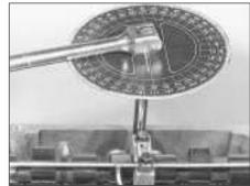
5B.52B Typical disc for angular tightening of cylinder head bolts
