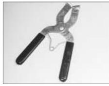
Piston ring removal/installation tool
