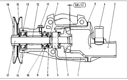
Fig. 2.4 Sectional view of 903 cc engine coolant pump (Sec 9)
