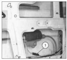
Fig. 9.11 Power-operated window motor (Sec 31)
