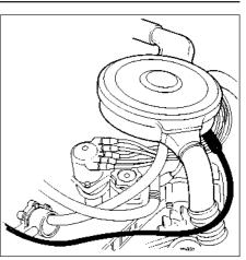
Fig. 3.9 Fuel return hose correctly located (Sec 8)
