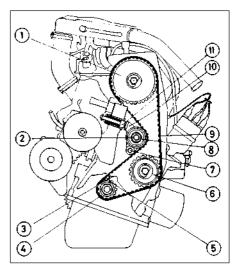
Fig. 1.29 Timing belt arrangement (Sec 28)
