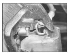
3.8B Cylinder body located on caliper bracket
