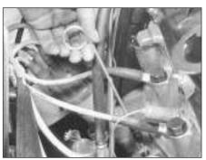
2.2 Withdrawing engine oil dipstick (1116 cc)
