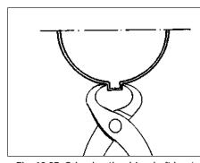
Fig. 13.97 Crimping the driveshaft boot securing band (Sec 13)
