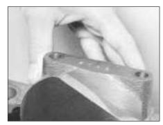
20.6 Fitting a main bearing cap
