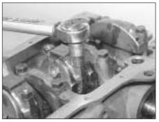
7B.197B . . . and tighten the nuts to the specified torque
