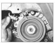
6B.19A Removing the TDC sensor
