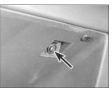
22.5A Facia fixing screw inside glovebox
