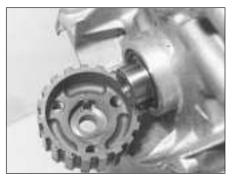
5D.16A Crankshaft sprocket showing integral key
