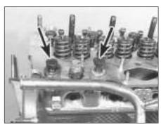
7.24B Cylinder head bolts holding coolant pipe
