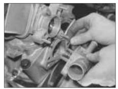
8C.31 Thermostat unit removal on the 1372 cc ie engine (distributor removed for clarity)
