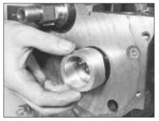
20.16B Camshaft front bearing
