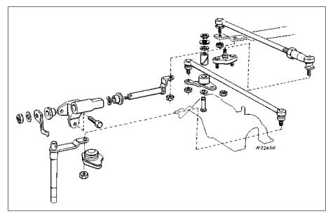
Fig. 13.91 Exploded view of the gear selector lever, rod and linkage components on 1372 cc models (Sec 12)
