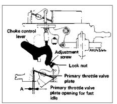
Fig. 3.25 Fast idle adjustment diagram (Weber 30/32 DMTR 90/250) (Sec 14) A = 0.90 to 0.95 mm (0.035 to 0.037 in)
