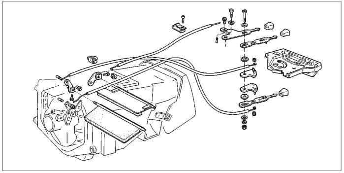
Fig. 2.12 Heater control components (Sec 13)
