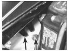
9C.55C Air cleaner casing lower bracket and bolt (arrowed)
