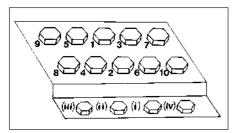
Fig. 13.13 Cylinder head bolt tightening sequence on the 1301 cc Turbo ie engine (Sec 6B)
