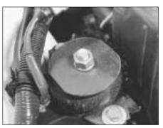
6B.16B Engine/transmission right-hand mounting
