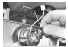
15.80B Roof-mounted spotlamp bulb removal
