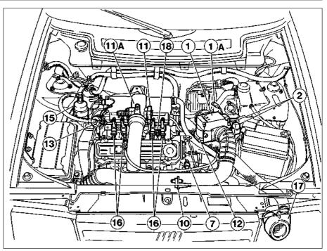
Fig. 13.49 Fuel injection system components layout in engine compartment on the 1372 cc Turbo ie engine (Sec 9E)
