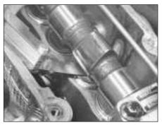
5B.1A Checking a valve clearance
