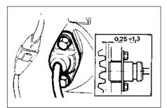
Fig. 4.10 Engine speed sensor gap (Sec 10)
