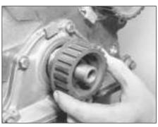
42.20 Fitting crankshaft timing belt sprocket
