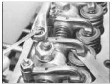
5.7 Adjusting a valve clearance
