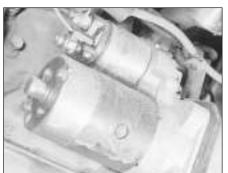
15.23B Starter motor and wiring connections on the 1372 cc ie engine
