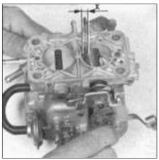
Fig. 3.22 Primary valve plate opening (Weber 30/32 DMTR 90/250) (Sec 14) X = 6.45 to 6.95 mm (0.25 to 0.27 in)
