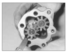
7B.176 Check gear-to-body clearance
