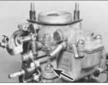
8.6 Carburettor mounting flange nut
