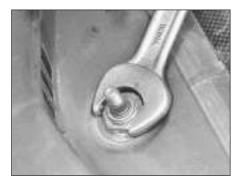
15.95 Unscrewing the wiper pivot nut
