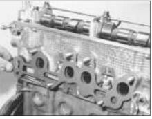
5D.25A Inlet manifold gasket
