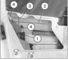
Fig. 9.13 Central door locking system components (Sec 32)
