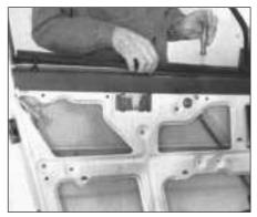
Fig. 12.7 Removing door weatherseal (Sec 12)
