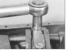
20.9 Tightening main bearing cap bolts
