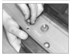
15.98A Remove the wiper motor retaining screws . . .
