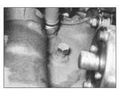
8C.9 Cylinder block drain plug
