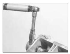
7B.85 Tightening a camshaft housing securing bolt
