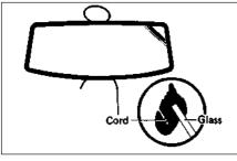
Fig. 12.17 Position of cord for fitting windscreen weatherseal (Sec 15)
