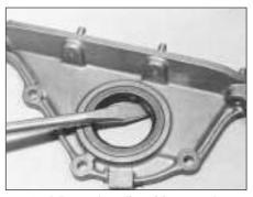
42.7A Removing oil seal from carrier
