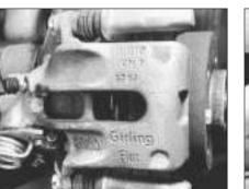
14B.23 Rear brake pad inspection aperture
