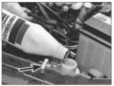
8C.28 Topping up the radiator coolant level on the 1372 cc ie engine. Note orientation of radiator retaining clip (arrowed)
