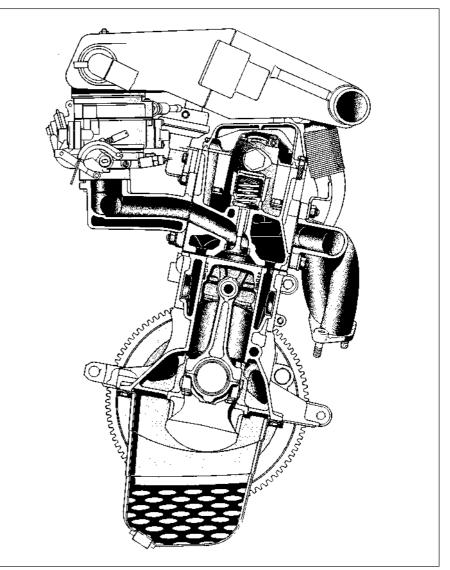
Fig. 13.2 Cross-section view of the 999 and 1108 cc engine (Sec 5A)
