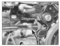
9B.36A Showing idle speed screw (arrowed) and . . .
