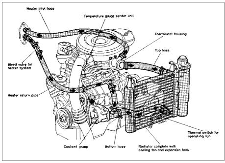
Fig. 2.1 Cooling system on 903 cc engine (Sec 1)
