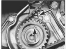
7B.50 Crankshaft at TDC with key and timing mark aligned (arrowed)
