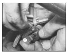
5B.32 Disconnecting the throttle cable
