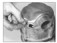
15.12B Alternator rear cover and fixing nut
