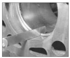
18.24B Checking piston ring end gap
