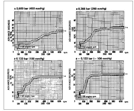
Fig. 13.79 Ignition advance curves - Microplex ignition system on the 1301 cc Turbo ie (Sec 10)
