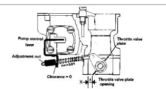
Fig. 3.11 Accelerator pump setting diagram (Weber 32 ICEV 50/250) (Sec 9)
