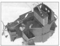
Fig. 2.10 Withdrawing heater matrix (Sec 13)
