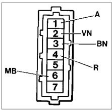
Fig. 13.81 Microplex ignition system control unit connection (Sec 10) For colour code, see main wiring diagrams
