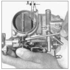
Fig. 3.20 Moving lean out valve rod (Solex C32 DISA 11) (Sec 10) X = 4.75 to 5.25 mm (0.187 to 0.207 in)
