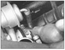
9F.17 Releasing turbocharger air hose clip
