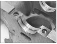
5D.2 Main bearing shell in crankcase
