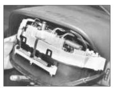
15.59A . . . withdraw the instrument panel . . .
