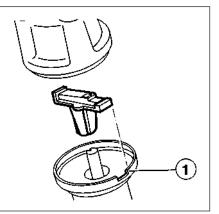
Fig. 13.85 Rotor arm must align with slot (1) in distributor housing when refitting distributor - Digiplex 2 ignition system (Sec 10)
