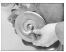
7B.34 Crankshaft pulley nut removal
