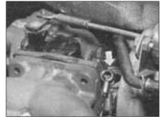
Fig. 13.64 Turbocharger oil supply pipe connection (arrowed) (Sec 9F)
