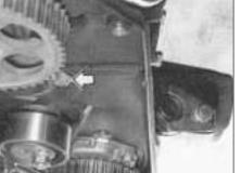
Fig. 13.18 Timing belt rear cover bolt (arrowed) - 1372 cc ie and Turbo ie engines (Sec 7B)
