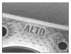
29.21A Cylinder head gasket top face marking
