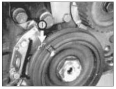
Fig. 1.28 TDC marks (1) at front of engine (Sec 28)
