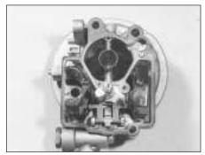
9B.23C Underside view of the cover on the Weber 32 TLF carburettor
