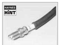
It's often difficult to insert spark plugs into their holes without cross-threading them. To avoid this possibility, fit a short piece of rubber hose over the end of the spark plug. The flexible hose acts as a universal joint, to help align the plug with the plug hole. Should the plug begin to cross-thread, the hose will slip on the spark plug, preventing thread damage.
