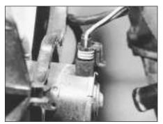
5C.19B Radiator fan motor wiring connector
