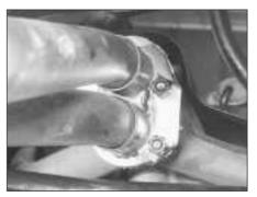
44.15 Exhaust downpipe flange nuts
