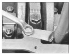
42.12 Tightening oil drain pipe bolt
