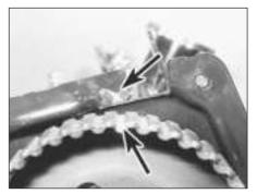
28.4 Camshaft sprocket alignment marks
