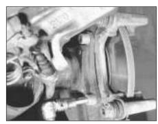
14B.42 Unscrewing a rear caliper bracket bolt
