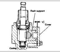
Fig. 10.5 Sectional view of rack damper (Sec 7)
