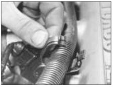
9C.77 Wiring loom clip and bracket
