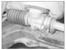
6.4 Steering rack housing at pinion end
