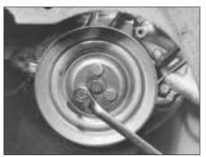
5B.7 Unscrewing the crankshaft pulley bolts
