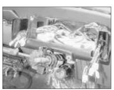
21.5 Instrument panel and steering wheel removed
