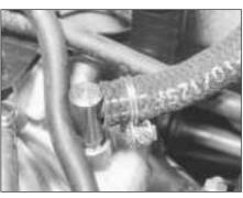
44.21B Brake servo hose at manifold
