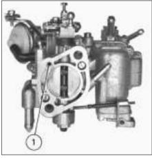
Fig. 3.14 Anti-flooding device vacuum intake (Weber 342 ICEV 50/250) (Sec 9) 1 Vacuum intake hole
