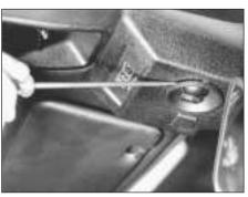
15.82 Roof-mounted clock retaining screw removal
