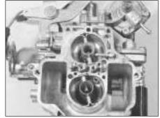
9B.34E Weber 30/32 DMTE carburettor from above (with cover removed)
