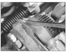
8C.53 Tightening the alternator adjuster nut
