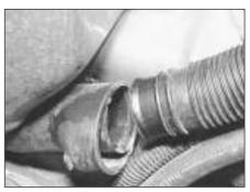
9A.5B Air cleaner cold air intake on the 999 cc model
