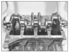
5D.4 Fitting the crankshaft
