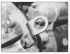
5D.38 Lifting eye on flywheel housing flange
