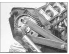
7B.48 Tightening the crankshaft sprocket bolt
