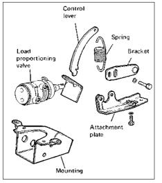
Fig. 8.9 Components of the pressure regulating valve (Sec 10)
