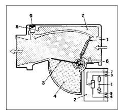
Fig. 13.39 Sectional view of airflow meter -1301 cc Turbo ie engine (Sec 9C)
