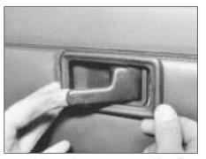
11.3A Removing remote control handle escutcheon
