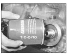
2.8 Screwing on the oil filter (903 cc)
