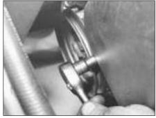
5B.6 Timing cover lower fixing bolt removal
