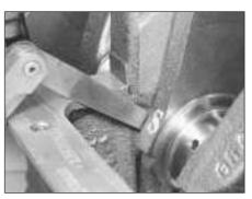
20.10 Checking crankshaft end float
