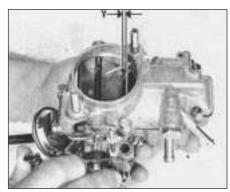
Fig. 3.15 Choke valve gap opening (Weber 32 ICEV 50/250) (Sec 9) Y = 3.75 to 4.25 mm (0.148 to 0.167 in)
