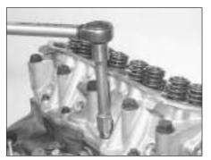
7B.122 Tighten the smaller cylinder head bolts to their specified torque setting
