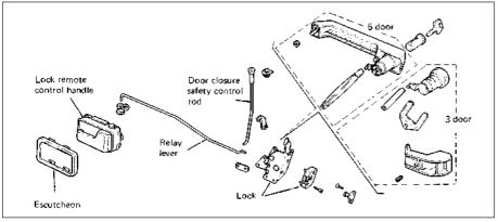
Fig. 12.15 Door lock components (Sec 12)
