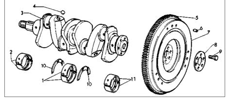
Fig. 1.24 Crankshaft and flywheel (Sec 16)
