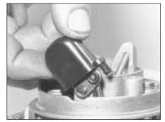
9B.23A Choke linkage cover removal from the Weber 32 TLF carburettor
