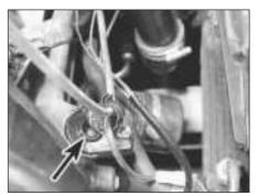
6B.22 Distributor drive hole cover plate (arrowed)
