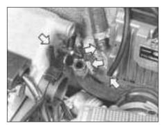
Fig. 13.57 Detach the vacuum pick-up pipes from the points arrowed on the 1372 cc Turbo ie engine (Sec 9E)
