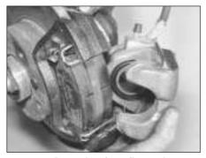
3.4 Removing the caliper unit
