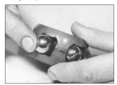
13.19A CV joint balls and cage
