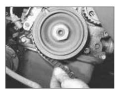
6B.19B Removing the timing belt
