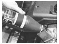
7A.11 Topping up the engine oil level -1372 cc engine
