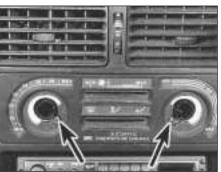
15.69A . . . undo the retaining screws (arrowed)
