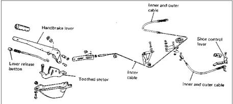
Fig. 8.13 Handbrake components (Sec 17)
