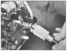
23.2 Speedometer cable connector at head
