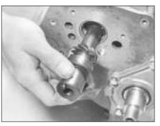
42.9 Fitting the auxiliary shaft
