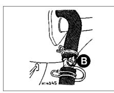
Fig. 2.2 Plug (B) in heater hose (Sec 2)
