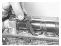
5B.52A Inserting a cylinder head bolt
