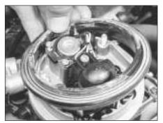
9D.39 Removing the filter seal from the injector unit
