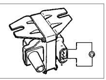
Fig. 13.83 Test connections for ignition coil primary windings check - Digiplex 2 ignition system (Sec 10)
