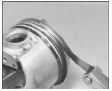
18.24A Checking piston ring groove clearance
