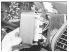
13.5A Withdrawing switch panel
