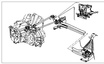
Fig. 13.89 Gearchange control linkage on the 1301 cc Turbo ie model with Antiskid (Sec 12)
