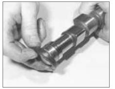
5B.26A Camshaft oil seal
