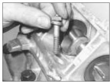
7B.77 Removing one of the camshaft housing shorter securing bolts
