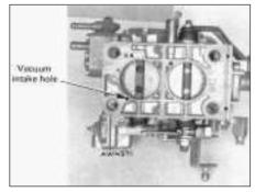
Fig. 3.31 Vacuum drilling for automatic anti-flooding device (Solex C30-32 CIC/1) (Sec 15)
