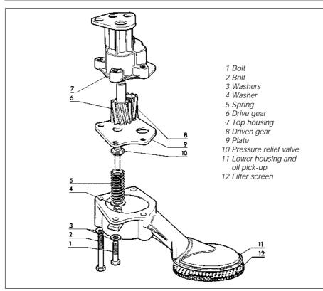
Fig. 1.27 Exploded view of oil pump (Sec 18)
