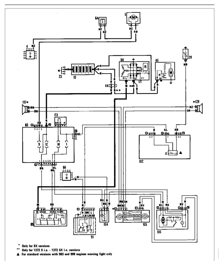
Wiring diagram 45 - radiator cooling fan, heater, radio and cigar lighter (1990-on 45, 55, 70 and 1.4 models)
