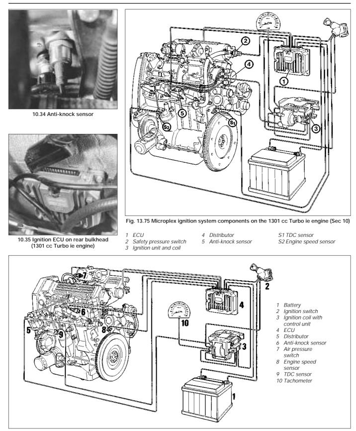
Fig. 13.76 Microplex ignition system components on the 1372 cc Turbo ie engine (Sec 10)
