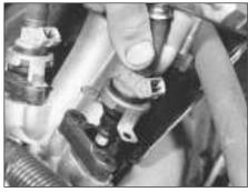
9C.80B Fuel injector removal
