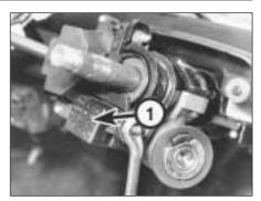
11.4 Unscrewing steering column switch clamp nut
