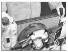
7.4B Removing radiator/fan assembly
