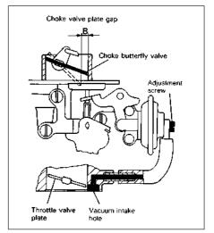
Fig. 13.38 Automatic anti-flooding device adjustment - Weber 32 TLF carburettor (Sec 9B)
