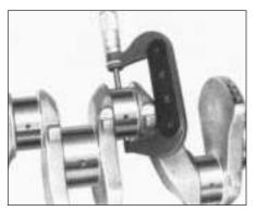
Fig. 1.25 Checking a crankpin (Sec 18)
