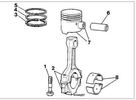
Fig. 1.8 Piston/connecting rod components (Sec 9)
