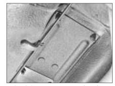
12B.15B Access cover to gear lever lower connection to rod on the 1372 cc engine
