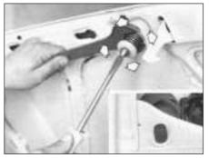
Fig. 12.2 Adjusting bonnet lock striker (Sec 8)
