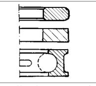
Fig. 13.5 Piston ring arrangement on the 999 cc engine (Sec 5B)
