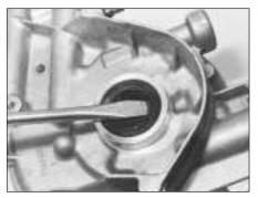
5B.77A Removing the oil pump seal
