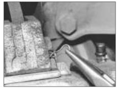
14A.2A Front brake pad locking block is secured by a clip on the inboard end of the brake unit on certain models
