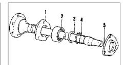
Fig. 13.98 Components of the intermediate driveshaft - Turbo ie models (Sec 13)
