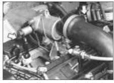
Fig. 13.55 Disconnecting the air intake duct and accelerator cable from the throttle housing on the 1372 cc Turbo ie engine (Sec 9E)
