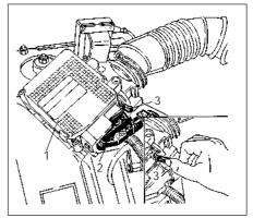
Fig. 13.62 ECU (1) wiring multiplug (2) and tag (3) - 1372 cc Turbo ie engine (Sec 9E)
