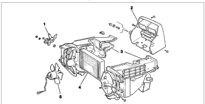
Fig. 13.34 Heater unit components on later models (Sec 8D)
