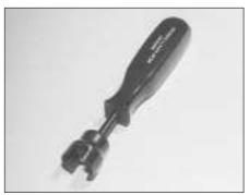
Brake shoe steady spring cup removal tool
