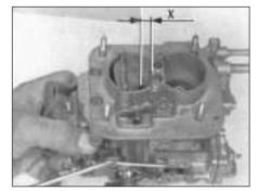
Fig. 3.32 Choke valve plate setting (Solex C30-32 CIC/1) (Sec 15) X = 4.75 to 5.25 mm (0.187 to 0.207 in)
