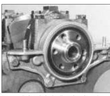
20.11B Crankshaft oil seal and carrier fitted
