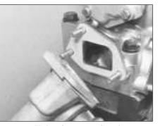
4.4 Fitting thermostat housing (1116 cc engine)
