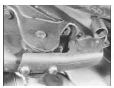
10.4 Pressure regulating valve bracket and tension spring
