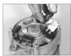
15.16B Removing the alternator brush holder
