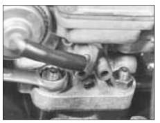
9B.37F Unscrewing a carburettor fixing nut
