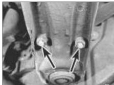
16.4 Anti-roll bar fixing nuts (arrowed)
