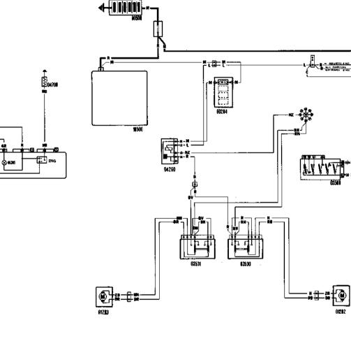
Wiring diagram 27 - electric windows (1301 cc Turbo ie model)
