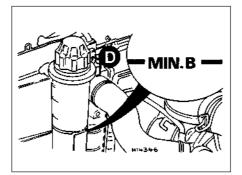
Fig. 2.3 Plug (D) in expansion tank (Sec 2)
