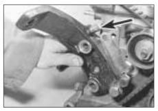
42.24C Engine mounting bracket with belt tensioner plunger (arrowed)
