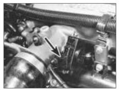
9C.90 Throttle position switch (wiring plug arrowed)
