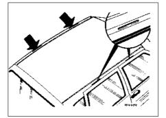
Fig. 12.22 Roof rack clamp locations (Sec 27)
