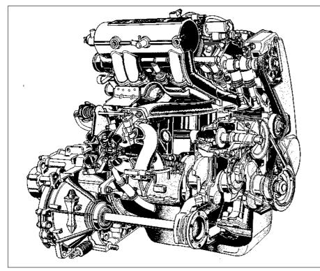
Fig. 13.10 Cutaway view of the 1301 cc Turbo ie engine (Sec 6A)
