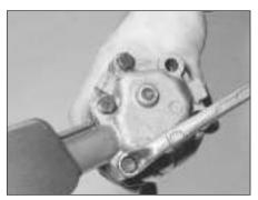
7B.171 Undo the oil pump cover bolts
