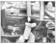
17.4 Throttle cable sleeve and bracket
