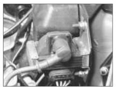
10.65 Ignition coil and connections on the 1372 cc ie engine
