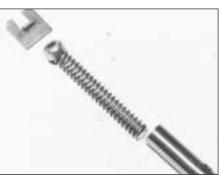
5B.72B Oil pump relief valve components
