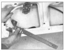
Fig. 12.10 Removing door window regulator (Sec 12)
