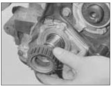
7B.47 Refitting the crankshaft sprocket
