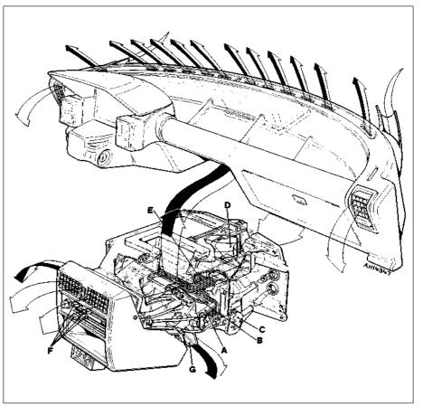
Fig. 2.7 Heater and ventilation system (Sec 11)
