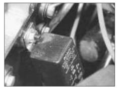
9C.84 Fuel injector system relay
