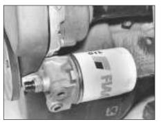
5D.29 Oil filter cartridge and mounting base
