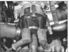
10.70 Ignition distributor and HT lead connections on the 1372 cc ie engine
