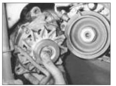
15.14 Withdrawing the alternator
