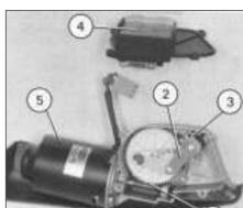
Fig. 9.6 Windscreen wiper motor components (Sec 25)
