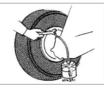
Fig. 8.12 Bleeding a rear wheel cylinder (Sec 12)
