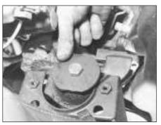
5C.31A Right-hand engine mounting disconnected
