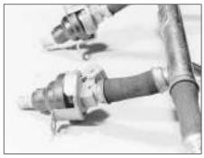
9C.81A Fuel injectors attached to fuel rail
