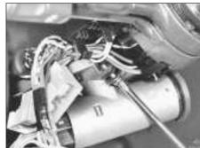
15.47A Undo the retaining screw . . .
