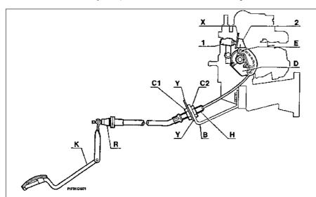
Fig. 13.47 Accelerator linkage and butterfly control lever - SPi models (Sec 9D)
