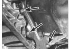
12B.33 Lower cover plate and retaining bolts (arrowed)
