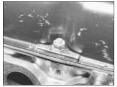
20.30 Rocker cover nut and thrust plate
