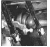
Fig. 1.16 Gearchange rods disconnected (Sec 13)
