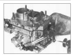
Fig. 3.29 Adjusting accelerator pump stroke (Solex C30-32 CIC/1) (Sec 15)
