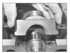
5D.6 Fitting a main bearing cap
