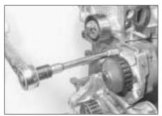
8A.17B Tightening the coolant pump bolts
