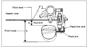
Fig. 3.10 Float setting diagram (Weber 32 ICEV 50/250) (Sec 9) A = 10.5 to 11.0 mm (0.41 to 0.44 in) B = 45.0 mm (1.77 in)
