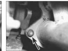
9F.16A Turbocharger-to-exhaust flange nut (arrowed)
