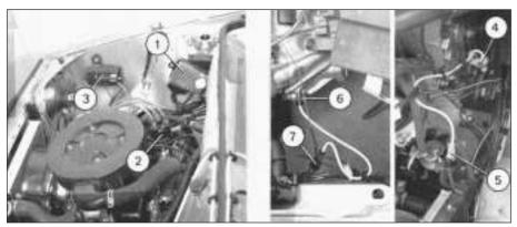
Fig. 4.8 Location of Digiplex ignition system components (Sec 9)
