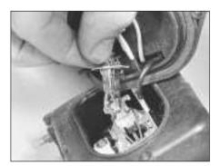
15.39 . . . detach the wires, extract the bulb
