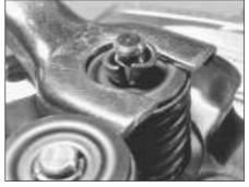
39.2 Valve spring compressor and split collets
