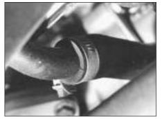
9F.20 Turbocharger oil return pipe at sump
