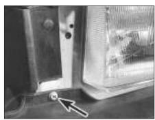
17.24 Front bumper upper mounting screw (arrowed)
