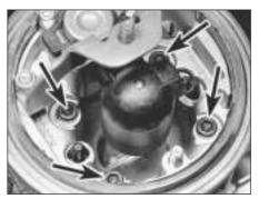
9D.44 Injector unit retaining screws (arrowed)
