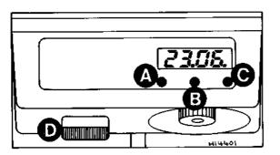
Fig. 9.16 Digital clock controls (Sec 35)
