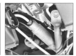
11.12 Clutch master cylinder and hydraulic pipe connections
