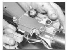
15.98C . . . and detach the wiring connector
