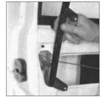
Fig. 12.13 Removing glass guide channel (Sec 12)
