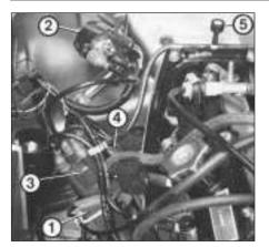
Fig. 13.71 Location of electronic ignition components on early models with breakerless ignition (Sec 10)
