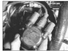
10.38 Removing the distributor cap
