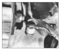
5C.24B Gearchange rod with ball socket connection
