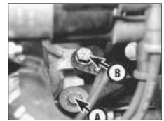
11.26 Clutch operating lever (A) and operating cylinder bracket-to-transmission housing bolt (B)
