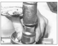
5B.77B Using a socket to fit the new oil pump oil seal
