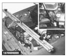
Fig. 13.93 FIAT lift beam/support bar in place to support the weight of the engine. Inset shows lift hook engagement point -1372 cc models (Sec 12)
