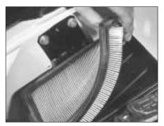
9C.27B Removing the air cleaner element
