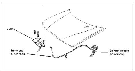
Fig. 12.1 Bonnet lock and release cable (Sec 8)
