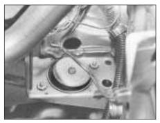
5B.107A Left-hand front engine/transmission mounting
