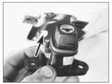
17.13 Tailgate handle link rod (arrowed)
