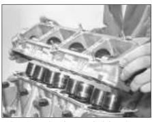
7B.84 Lowering the camshaft housing on to the cylinder head
