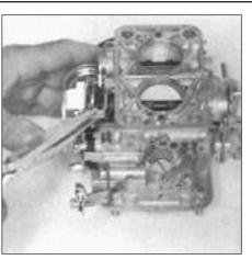
Fig. 3.23 Bending throttle lever stop (Weber 30/32 DMTR 90/250) (Sec 14)
