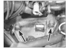
12B.36 Transmission upper retaining bolts. Note bracket under the left-hand bolt
