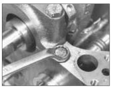
20.17 Camshaft front bearing lockscrew
