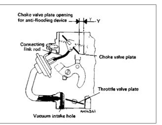
Fig. 3.13 Anti-flooding device (Weber 32 ICEV 50/250) (Sec 9)
