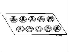
Fig. 1.30 Cylinder head bolt tightening sequence (Sec 29)
