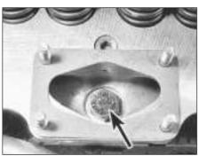
7.24A Cylinder head bolt in intake manifold
