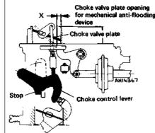
Fig. 3.26 Anti-flooding device (mechanical) adjustment diagram (Weber 30/32 DMTR 90/250) (Sec 14) X = 7.0 to 7.5 mm (0.28 to 0.30 in)
