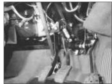
14B.47 Right-hand end of brake pedal cross-shaft
