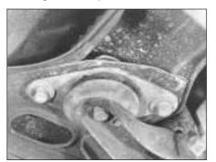
5B.107B Left-hand rear engine/transmission mounting
