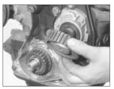
7B.45 Withdrawing the auxiliary shaft sprocket
