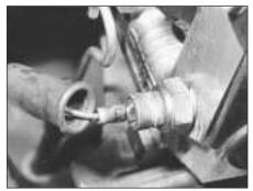
5C.16 Coolant temperature switch
