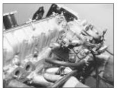
19.4C Fitting intake manifold complete with carburettor
