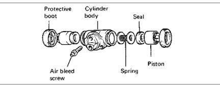
Fig. 8.4 Exploded view of a rear wheel cylinder (Sec 7)
