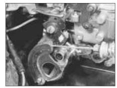
9B.37B Throttle cable connection on the Weber 30/32 DMTE carburettor
