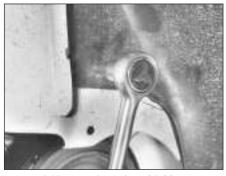
10.4A Unscrewing wing shield screw
