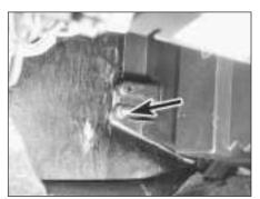
12.10 Heater lower mounting bolt
