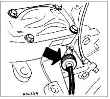
Fig. 1.11 Speedometer drive cable at transmission (Sec 13)
