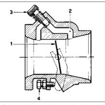
Fig. 13.40 Sectional view of throttle valve housing - 1301 cc Turbo ie engine (Sec 9C)
