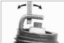
Adjusting spark plug gap
