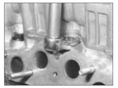
29.13 Using a crowfoot type wrench on a cylinder head bolt
