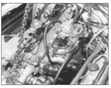
44.8A Raising engine/transmission into engine compartment
