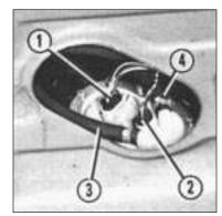
Fig. 13.63 Fuel pump and sender unit location on the 1372 cc Turbo ie engine (Sec 9E)
