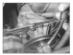
8C.40 Coolant pump/alternator bracket bolt removal
