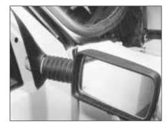
24.4 Withdrawing exterior mirror and trim plate
