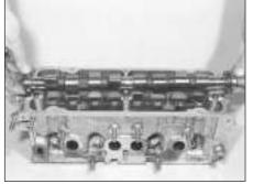
5B.23C Camshaft lubrication pipe
