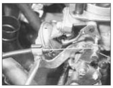
18.2 Choke cable at carburettor
