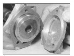
27.13A Removing camshaft end cover
