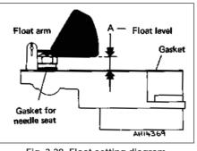
Fig. 3.28 Float setting diagram (Solex C30-32 CIC/1) (Sec 14)
