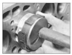
32.14 Fitting piston into cylinder bore
