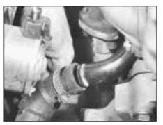
5C.7A Radiator hose connection to coolant distribution tube
