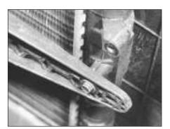
8C.22 Cooling fan to radiator securing bolt
