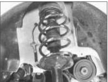
3.5 Withdrawing a front strut
