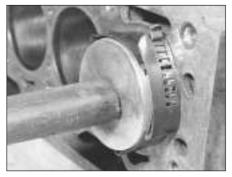
9.19 Fitting a piston/connecting rod
