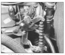
5C.12 Choke cable connection at carburettor
