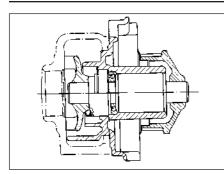
Fig. 13.28 Sectional view of the coolant pump on the 999 and 1108 cc engines (Sec 8A)
