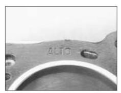
5B.50B Cylinder head gasket top surface marking
