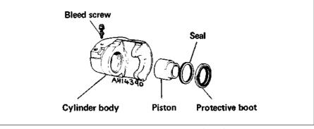
Fig. 8.2 Exploded view of caliper (Sec 5)
