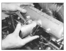
9C.73 Removing the inlet manifold
