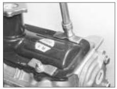
42.26 Tightening a camshaft carrier cover nut
