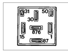
Fig. 13.43 System control relay connector plug terminals 1301 cc Turbo ie engine (Sec 9C)
