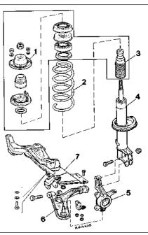
Fig. 11.3 Front strut components (Sec 3)
