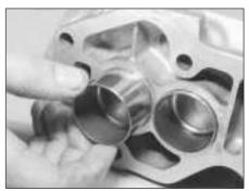
39.10 Cam followers fitted to camshaft carrier
