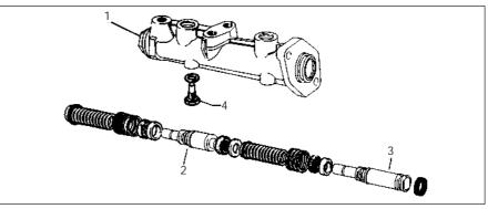
Fig. 8.6 Exploded view of master cylinder (Sec 9) 1 Cylinder body 2 Secondary piston 3 Primary piston 4 Stop bolt
