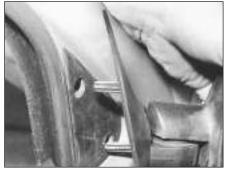
17.7B Withdrawing the exterior mirror
