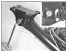
Fig. 11.9 Removing trailing arm pivot bolt (Sec 10)
