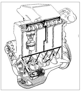
Fig. 13.4 999 and 1008 cc engine lubrication system (Sec 5A)
