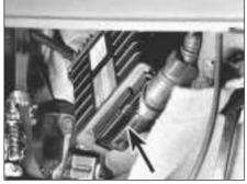
9D.58A Detach the multiplug (arrowed) . . .
