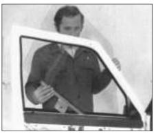
Fig. 12.8 Removing door glass (Sec 12)
