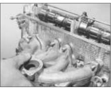
5D.25B Fitting the inlet manifold
