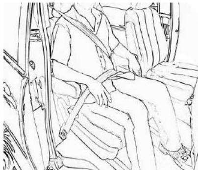
To fasten the seat belt when an outer armrest is used, arrange the shoulder belt above the armrest and the lap belt under the armrest.
