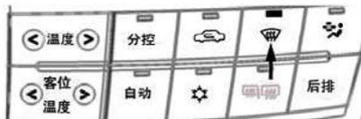
Under AUTO mode, the
