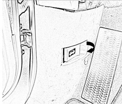
1. Pull the engine hood release handle and the hood will pop up slightly.
