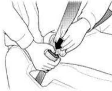
To release the seat belt, press the buckle release button and let the belt retract.
