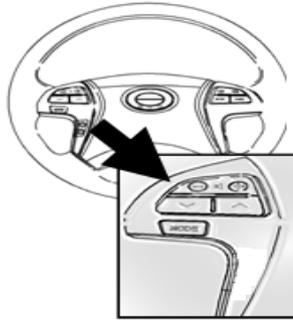
There are 3 buttons on the left of the steering wheel hub for setting the sound system. You can operate the basic functions of the sound system without getting your hands away from the steering wheel.
