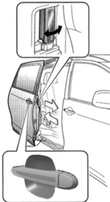
Open: pull the door handle outwards to unlock it and then slide it backward. Fully open the sliding door and it will be locked up by the positioning lock at the bottom.
