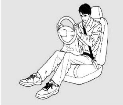
The frontal airbags deflate immediately after inflation, so they won't interfere with the driver's visibility or the ability to steer or control the vehicle.
