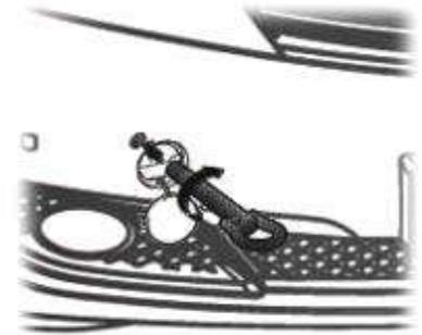
2. Get the front tow hook on hand. Install the front tow hook into the hole on the front bumper by rotating it clockwise (see "If You Have a Flat Tire" for the storage location of the toolkit).
