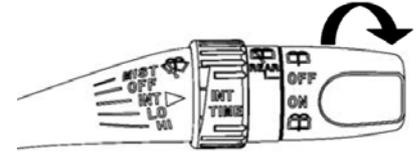
Rotate the knob on the control lever to turn on the rear windshield wipers.
