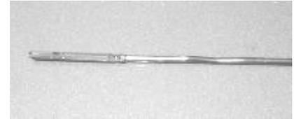
The upper and lower limits of the BYD483QB engine dipstick are indicated with two lines: F (Full) and L (Low). The oil level must fall between the upper and lower lines.
