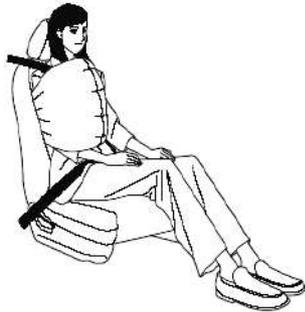
Side airbags, if equipped in the front seats, inflate in moderate to severe side collisions to protect the head and chest of the driver and front passenger from striking interior objects such as a window.
