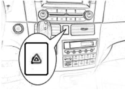
Press the switch shown in the figure to turn on the hazard warning flashers.
