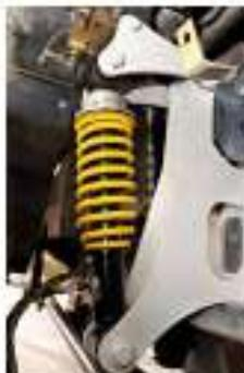
Technical innovation combines with new cab suspension system geometry to guarantee optimal driving comfort and the preloading adjustment feature provides a customized response to the various conditions of use.
