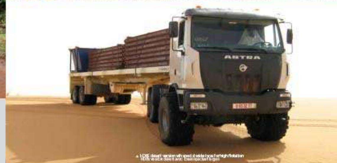
▲ HD8 chassis version with speed selection box for high rotation 1000 rpm via stick drive & lever. Diesel particulate filter
